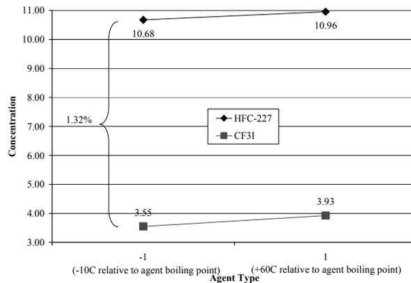
**Figure 7. Effect of Agent Type and Relative Temperature on Extinguishing Concentration.**
