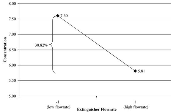
**Figure 12. Variability in Peak Concentration Required Due To Extinguisher Flow Rate.**
