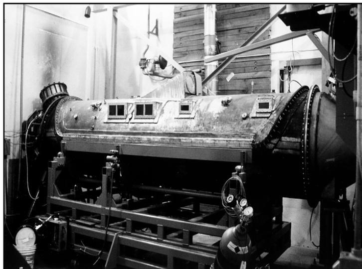
**Figure 1. Reconfigurable Nacelle Test Fixture in AENTF.**
