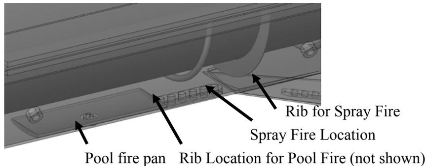
**Figure 2. Semi-Transparent View of Components in Fire Section of Fixture.**
