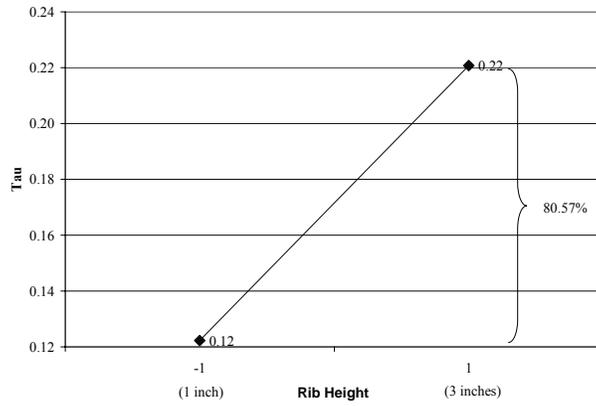
**Figure 9. Influence of Flame Stabilizing Rib Height on Value of Tau.**
