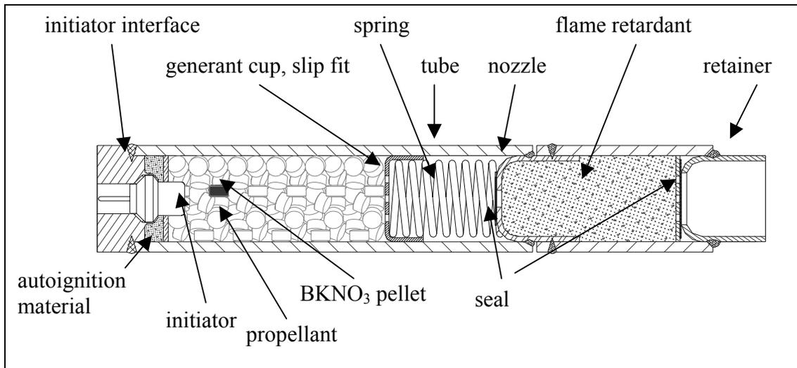
**Figure 1. Final design of gas generator housing configuration.**
