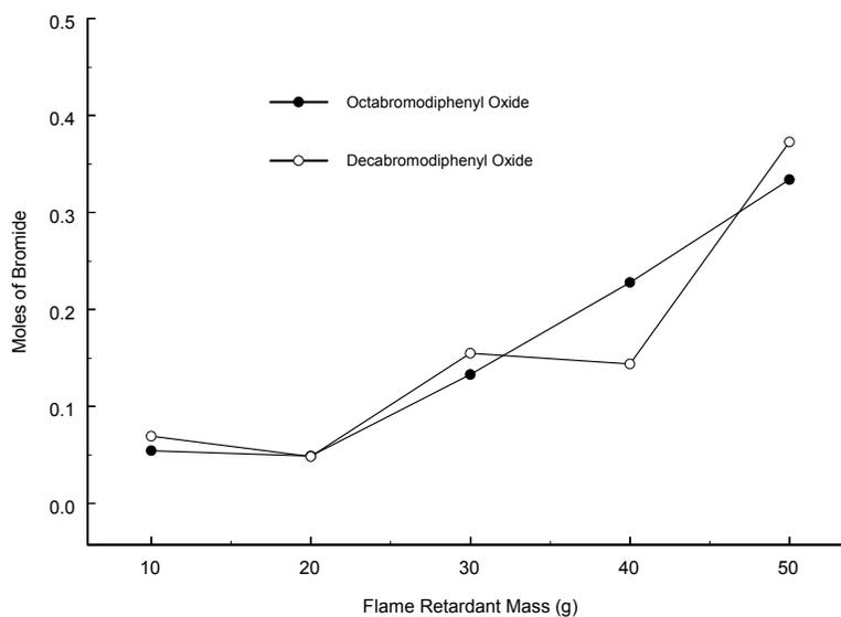
**Figure 3. Moles of gas-phase bromide formed versus amount of flame retardant.**
