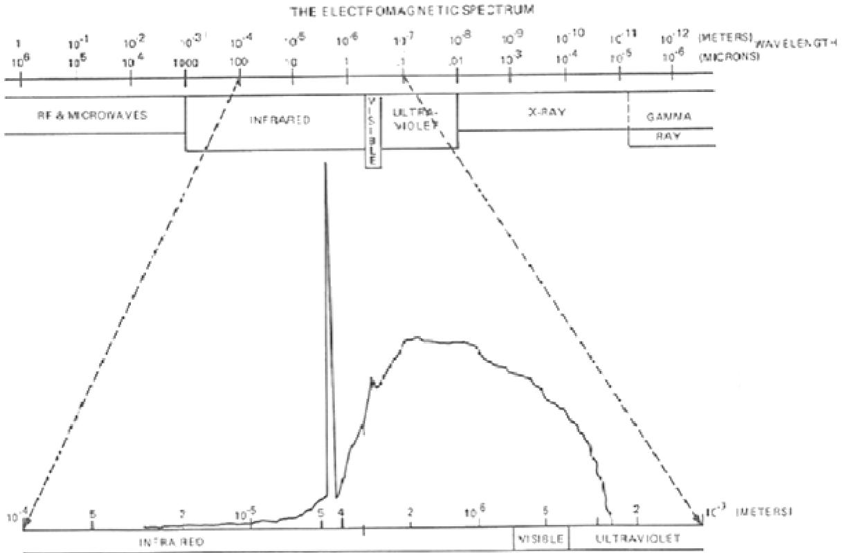
Figure 4. Electromagnetic spectrum for hydrocarbon fires.
