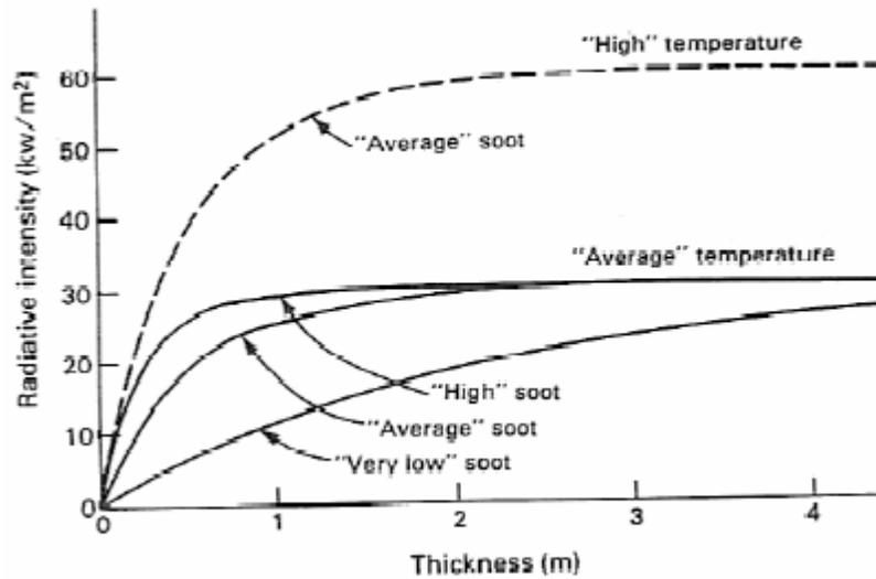
**Figure 2. Radiation intensity effects of temperature, flame thickness, soot levels.**
