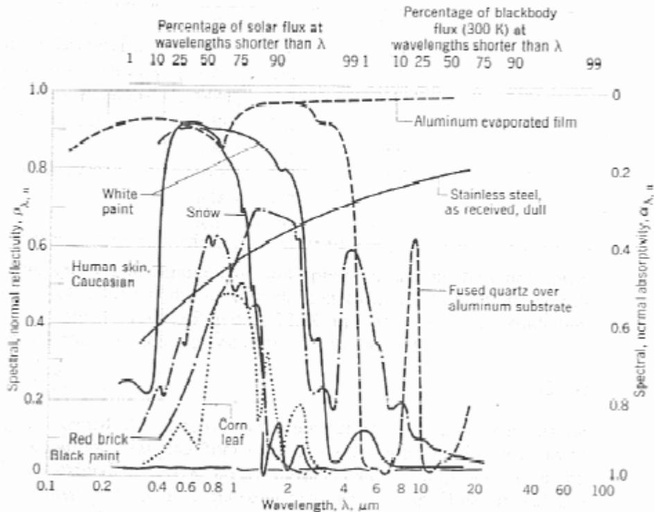
**Figure 3. Thermal Absorptivity Vs. Wavelength for Various Materials.**
