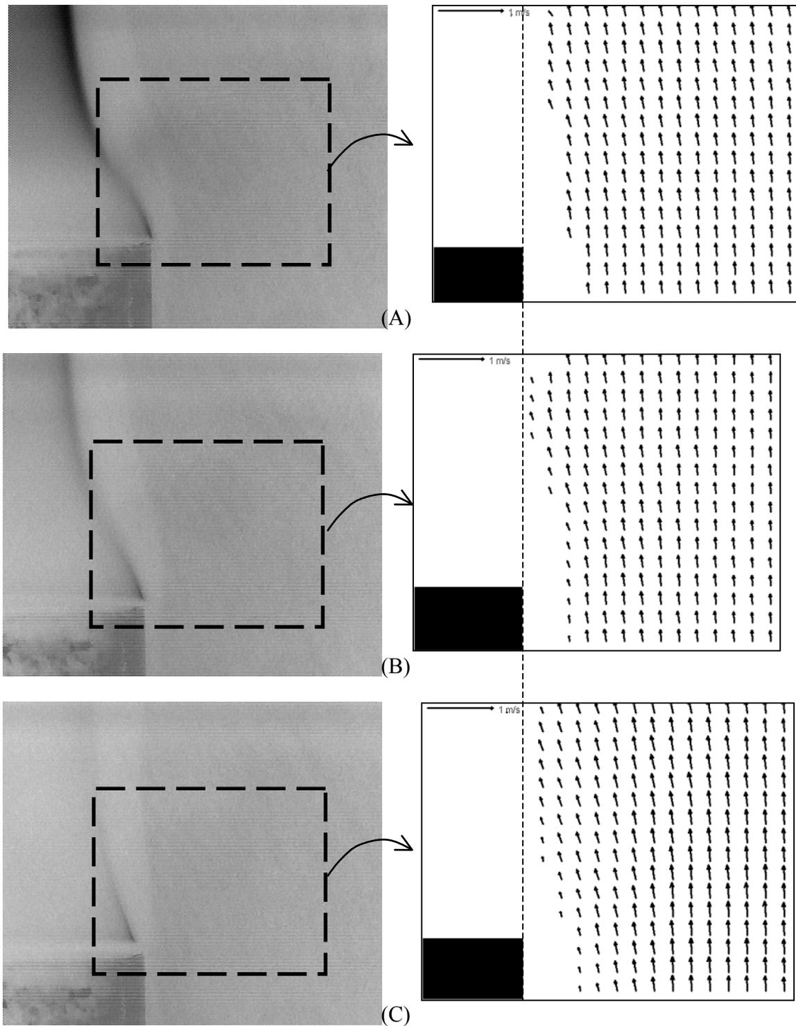
**Figure 3. Visual images (left) and PIV vector fields (right) for each of the three propane flame conditions. The location of the edge of the cup is indicated in the lower left by the black rectangle. The vector scale (1 m/s) is shown in the upper left of each PIV image.**
