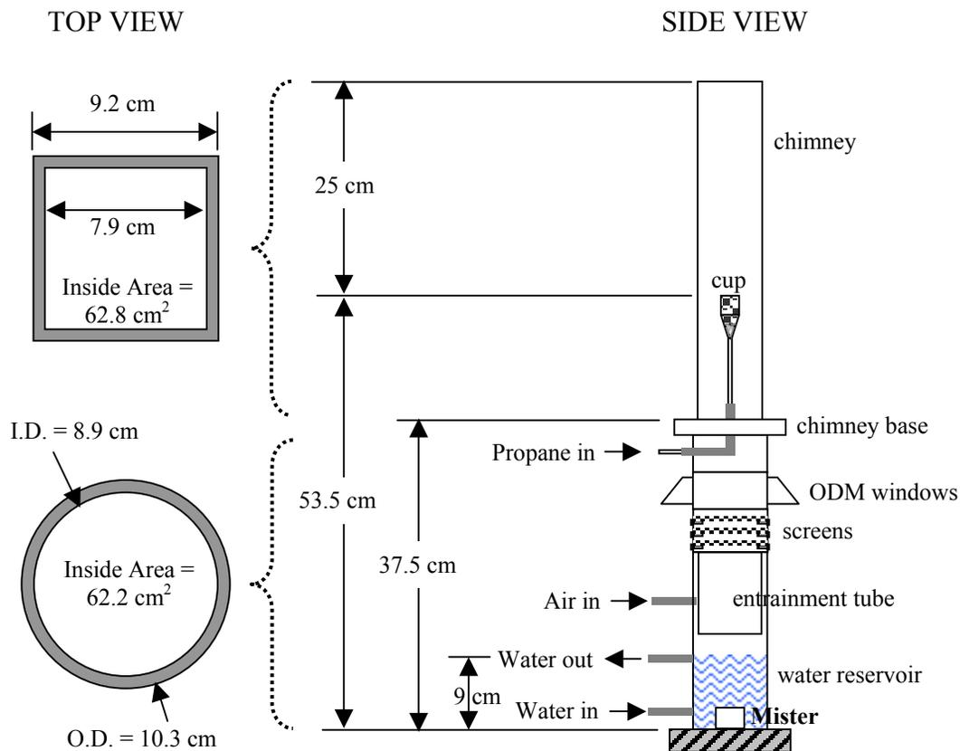
**Figure 1. The experimental cup burner apparatus. Top views of the lower enclosure sections and the chimney (not to scale) are shown on the left.**
