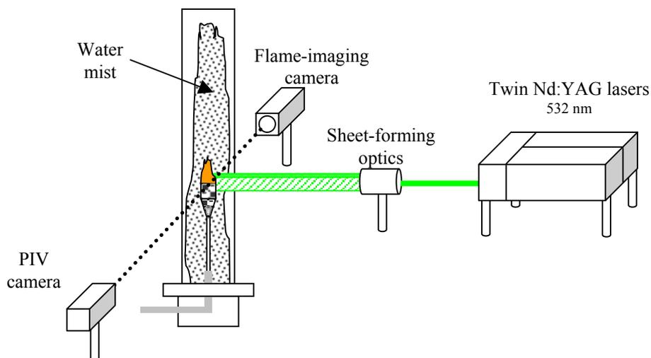
**Figure 2. Experimental configuration for flame and flow field imaging experiments.**
