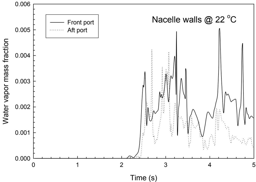
**Figure 3. Temporal variation of water vapor at the two measurement locations resulting from the injection of 416 L/min of liquid water at 1.5 s into a 22 °C inlet air flow with a speed of 4.25 m/s. The nacelle walls were at 22 °C.**
