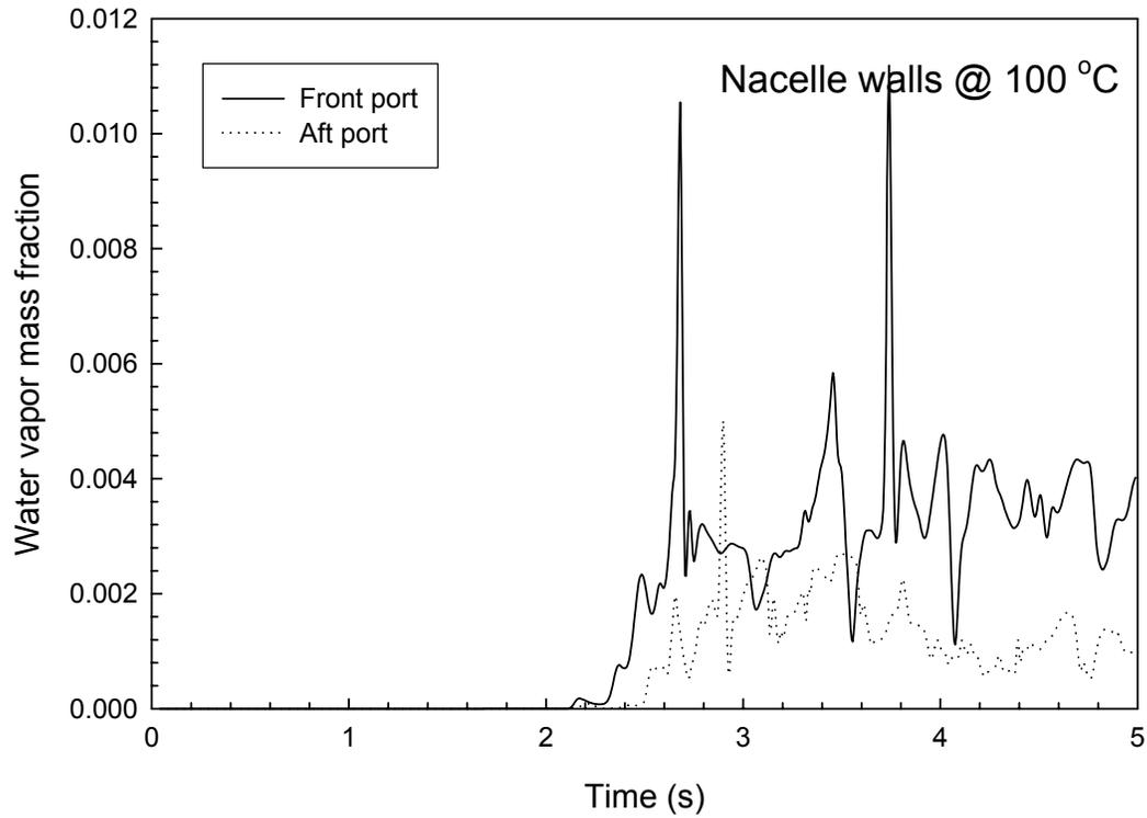
**Figure 4. Temporal variation of water vapor concentration at the two measurement locations resulting from the injection of 416 L/min of liquid water at 1.5 s into a 22 °C inlet air flow with a speed of 4.25 m/s. The nacelle walls were at 100 °C.**
