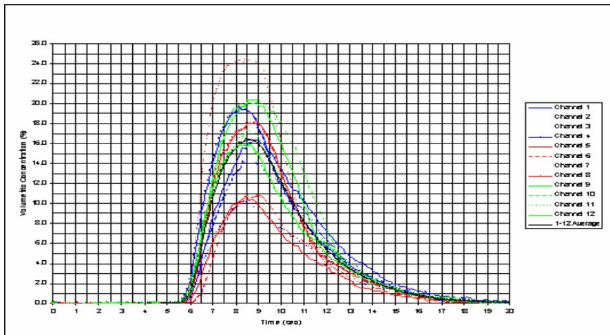
**Figure 1 HFC-125 Transient Injection Test Results**
