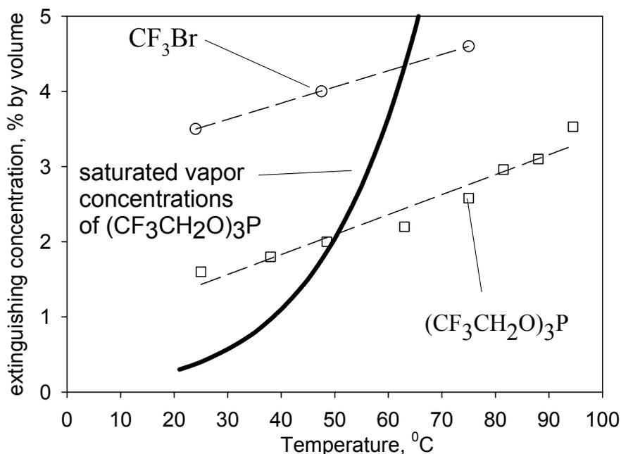
**Fig. 4. The dependencies of extinguishing concentration of  $\text{CF}_3\text{Br}$  and  $(\text{CF}_3\text{CH}_2\text{O})_3\text{P}$  obtained using cup burner on temperature of extinguishing mixtures (air + fire suppressant).**
