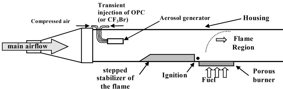
**Fig. 1. A scheme of Transient Application, Recirculating Pool Fire (TARPF) Apparatus.**
