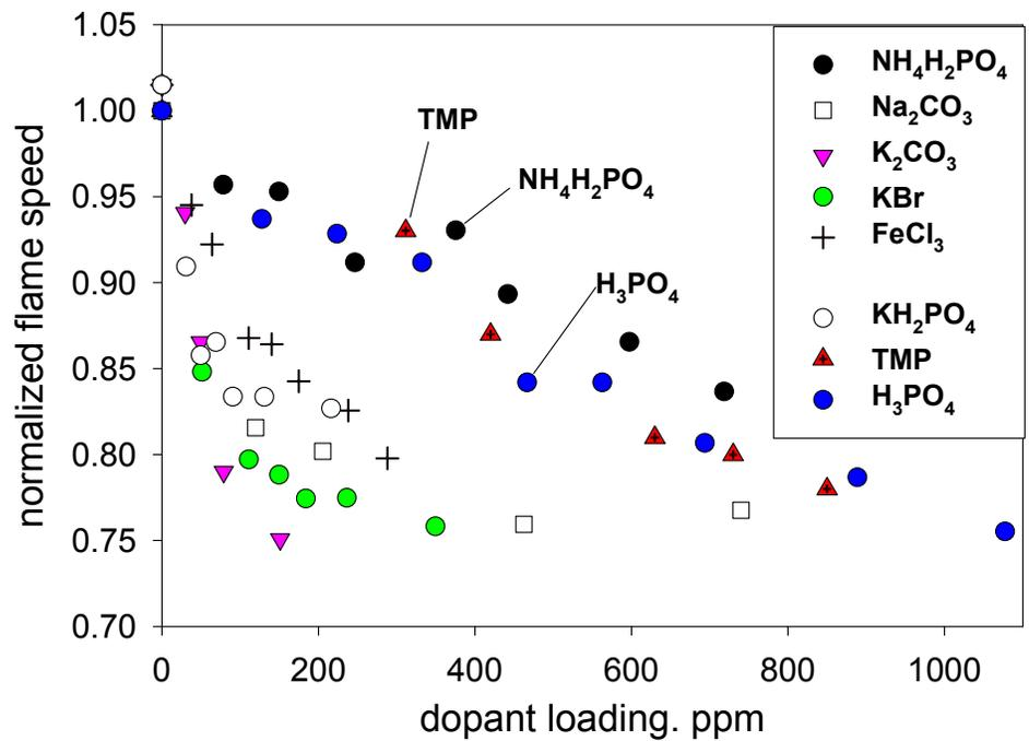
Fig. 2. Normalized speed of a stoichiometric premixed  $\text{C}_3\text{H}_8/\text{air}$  flame as a function of the dopants loading.
