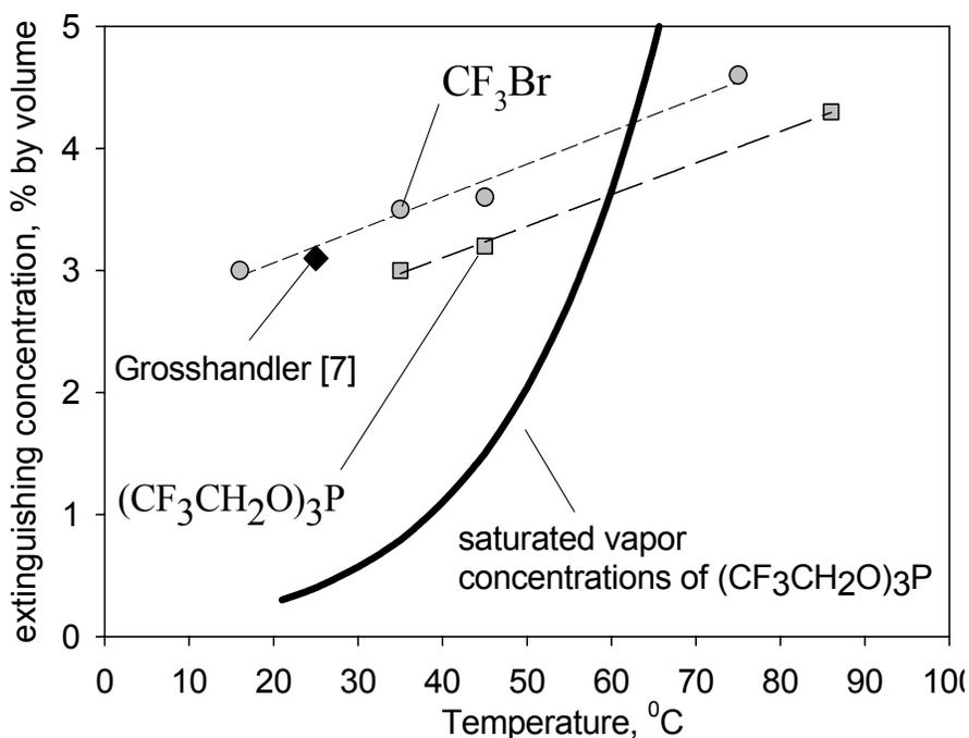
**Fig. 5. The dependencies of extinguishing concentration of  $\text{CF}_3\text{Br}$  and  $(\text{CF}_3\text{CH}_2\text{O})_3\text{P}$  obtained using TARPf apparatus on temperature of extinguishing mixtures (air + fire suppressant).**
