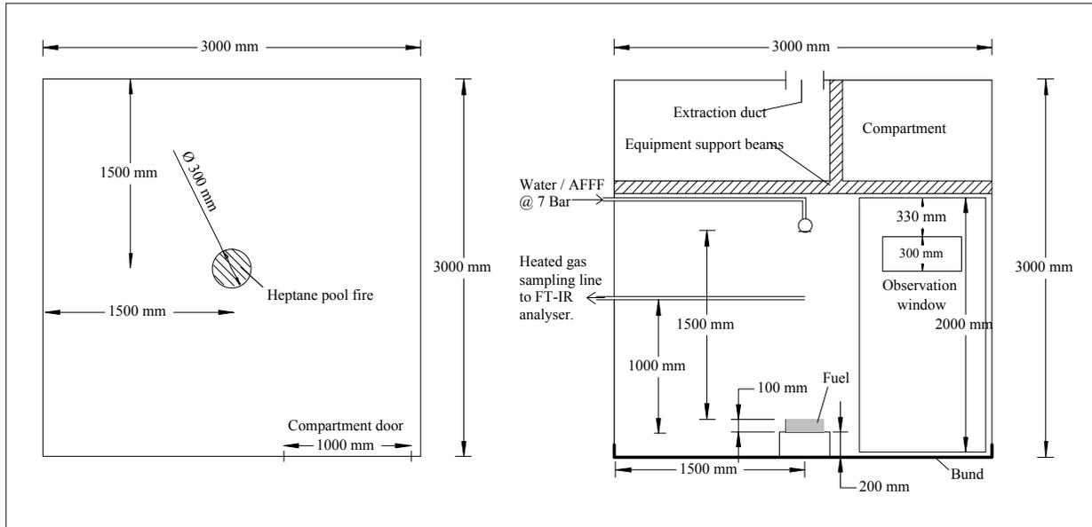
**Figure 1. Schematic of 3m cube for determination of the degradation products of additives**
