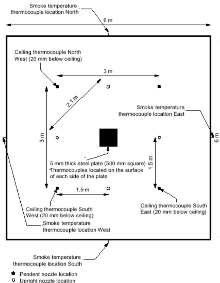
**Figure 7. Plan of ADD rig ceiling for deckhead cooling tests**
