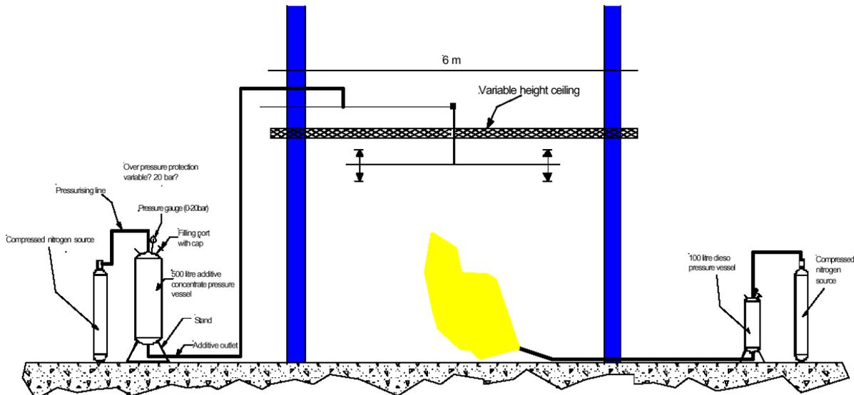
Figure 6. Elevation of ADD test rig
