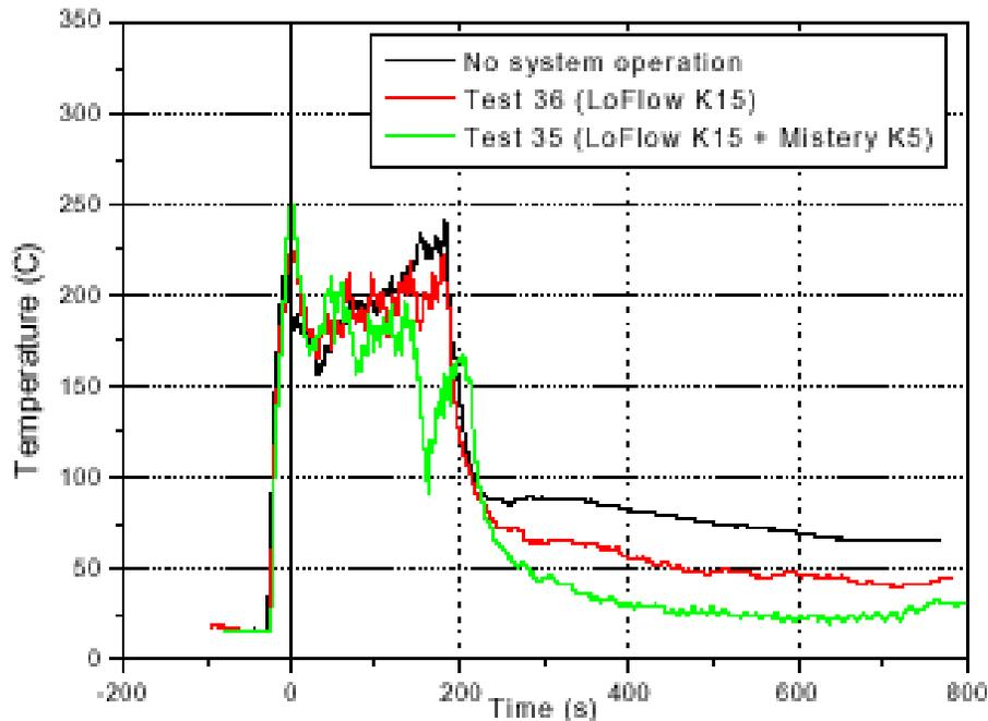
Figure 8. Steel plate temperatures on fire side
