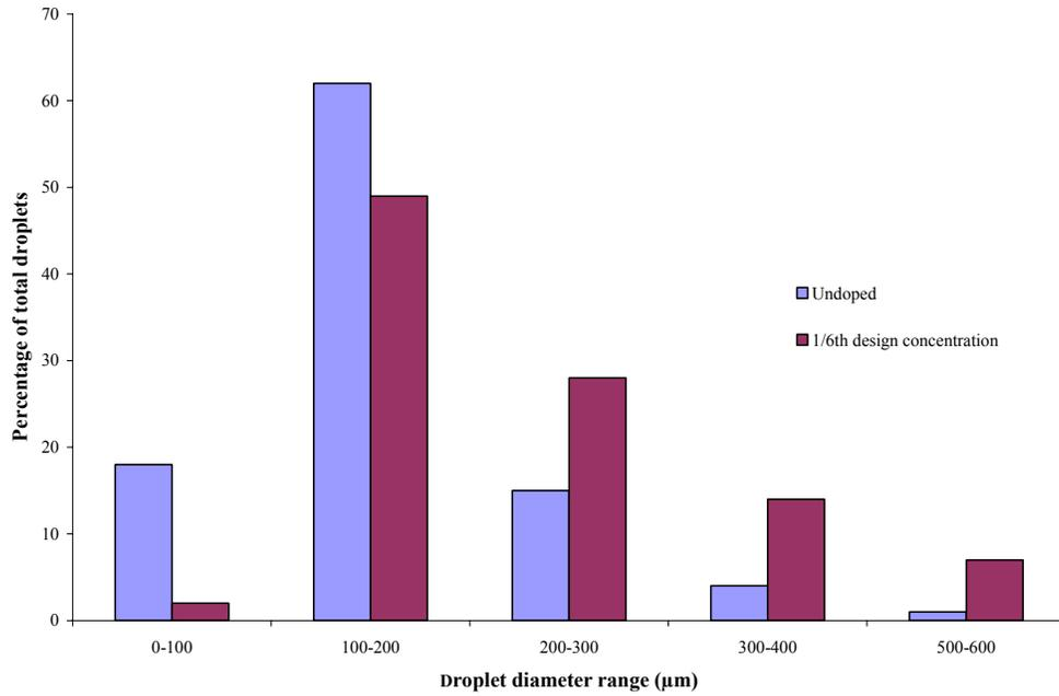
**Figure 4. Droplet diameters for Lechler 460.408.17CA nozzle**
