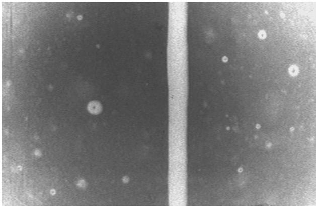
**Figure 2. Photograph of droplets from Lechler 460.408.17CA nozzle with water only**
