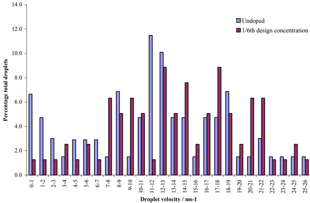
**Figure 5. Droplet velocity for Lechler 460.408.17CA nozzle**
