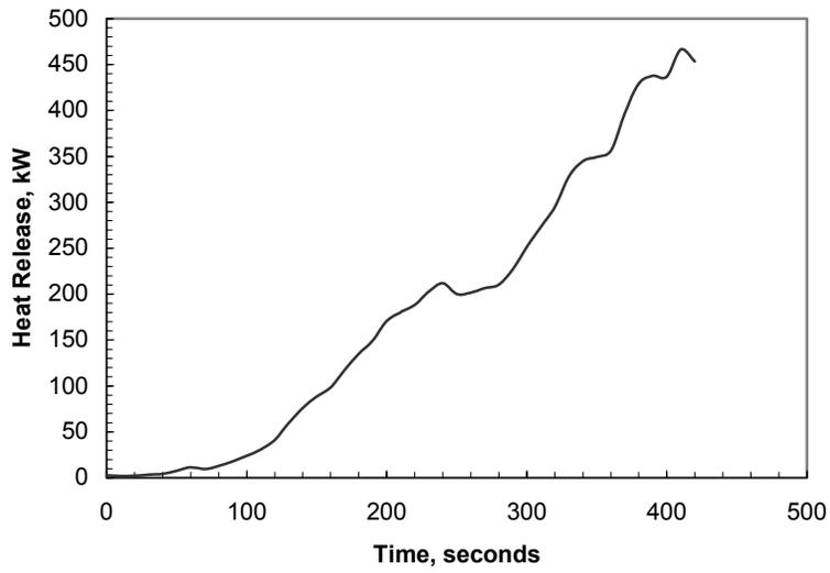
**Figure 3. Heat Release Rate for In-Cabinet Test Fire**
