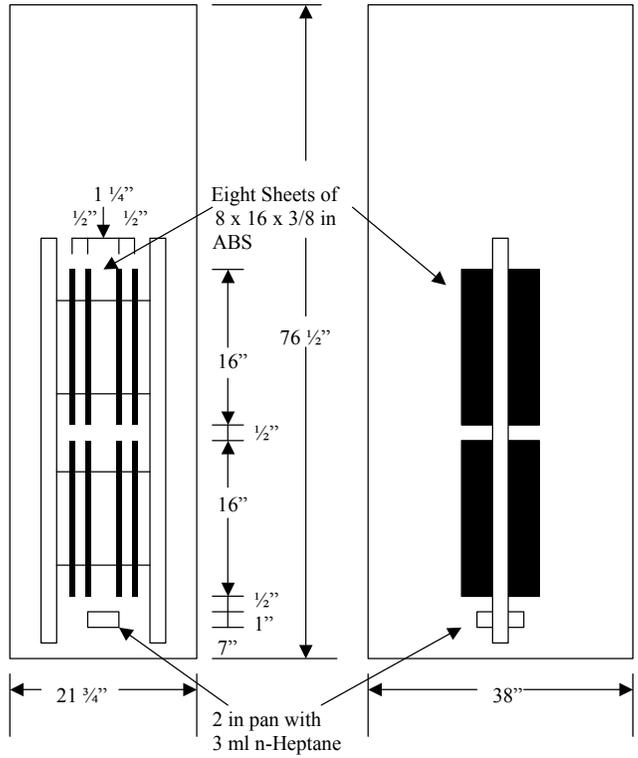
**Figure 2. Fuel Array Schematic**
