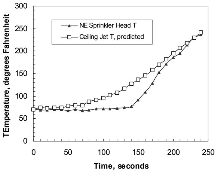
**Figure 5. Ceiling Jet Temperature at Northeast Sprinkler Head**
