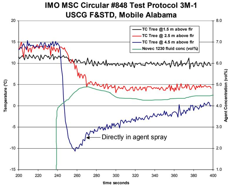
**Figure 2: Actual 500m<sup>3</sup> Room Discharge Temperature Profile**
