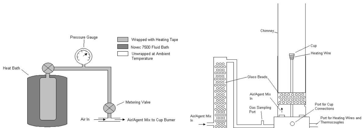
**Figure 4: Agent/air supply to cupburner apparatus**
