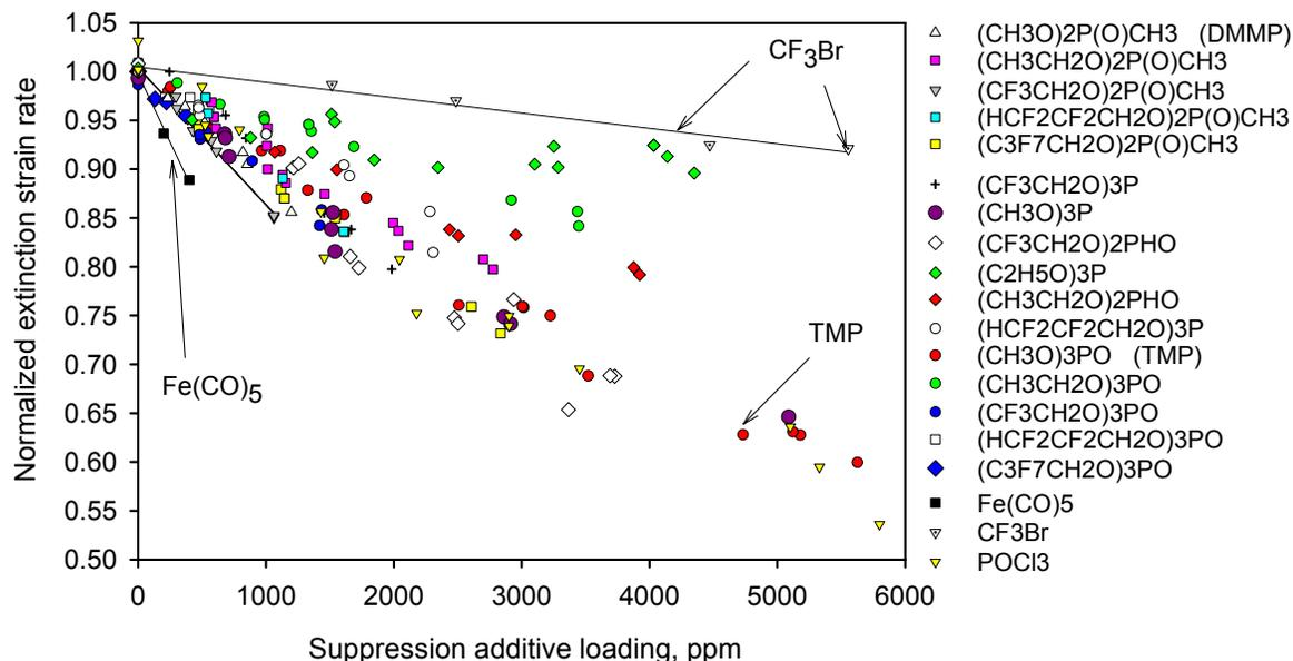
**Fig.2. Normalized extinction strain rate of the flame as a function of OPC and other suppression additives loading**
