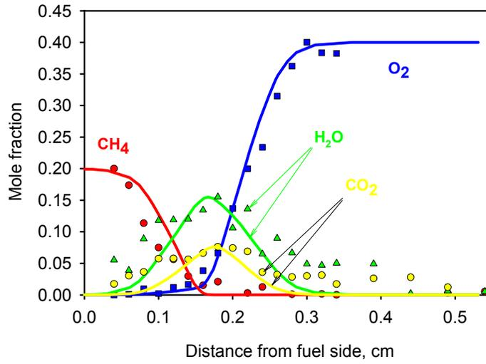
**Figure 5. Concentration profiles in diffusion counterflow CH<sub>4</sub>/N<sub>2</sub> – O<sub>2</sub>/N<sub>2</sub> flame. Symbols – experiment obtained with MBMS system - sampling at the distance 3 mm from the burner axis , line - modeling - along the burner axis**
