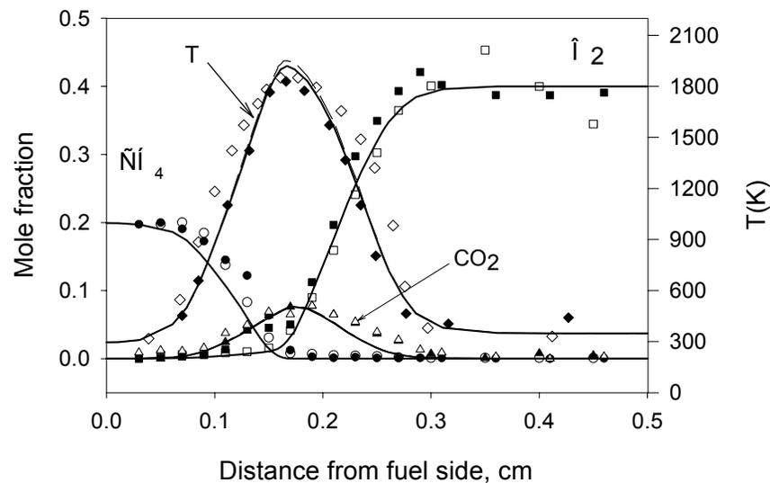
**Fig. 4. Concentration and temperature profiles in diffusion counterflow  $\text{CH}_4/\text{N}_2 - \text{O}_2/\text{N}_2$  flame doped with 1200 ppm TMP (filled symbols – experiment – microprobe sampling at the distance 3 mm from the burner axis, dashed line - modeling) and without additive (open symbols – experiment, solid lines - modeling). Strain rate is  $358 \text{ s}^{-1}$**
