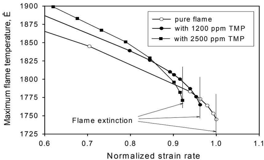
**Fig. 3. Calculated dependence of a maximum flame temperature (pure and doped) vs normalized global strain rate. Potential flow boundary conditions**
