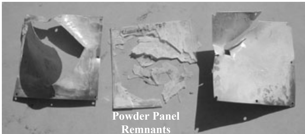
Figure 5. Entire Contents of Enhanced Powder Panel Released and Fire Prevented
