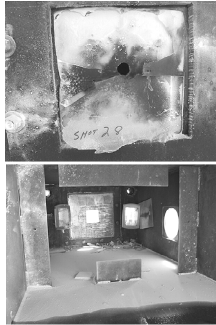
Figure 3. Comparison Of Commercial And Enhanced Powder Panel Agent Release In JTCG/AS Dry Bay Fire Extinguishing Testing
