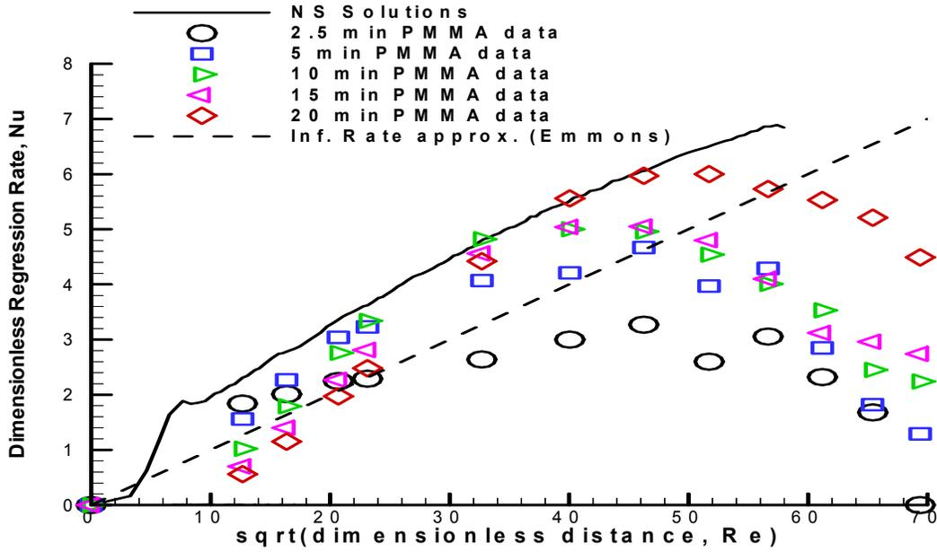
**Figure 4 Comparison of Steady State NS Solutions and BL theory with PMMA Experiments Performed for Different Burn Times and at Fixed  $U=84$  cm/sec**
