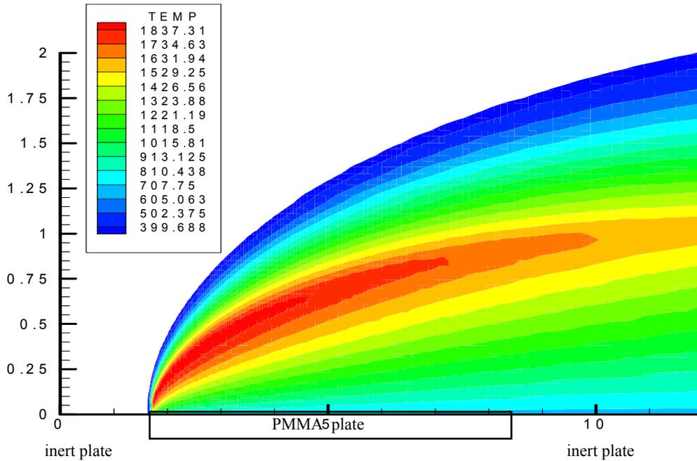
**Figure 1 Navier-Stokes (NS) Solutions for Temperature Contours for  $U=60 \text{ cm/sec}$**
