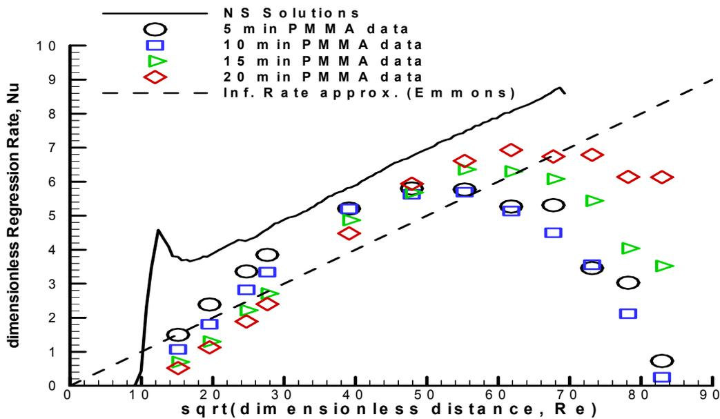
**Figure 5 Comparison of Steady State NS Solutions and BL theory with PMMA Experiments Performed for Different Burn Times and at Fixed  $U=120$  cm/sec**
