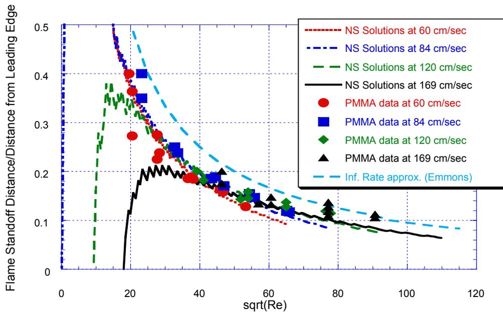
**Figure 2 Comparison of NS Solutions for Flame Standoff Distance with PMMA data and the Classical Boundary Layer (BL) Theory Given by  $10.0/\sqrt{Re}$**
