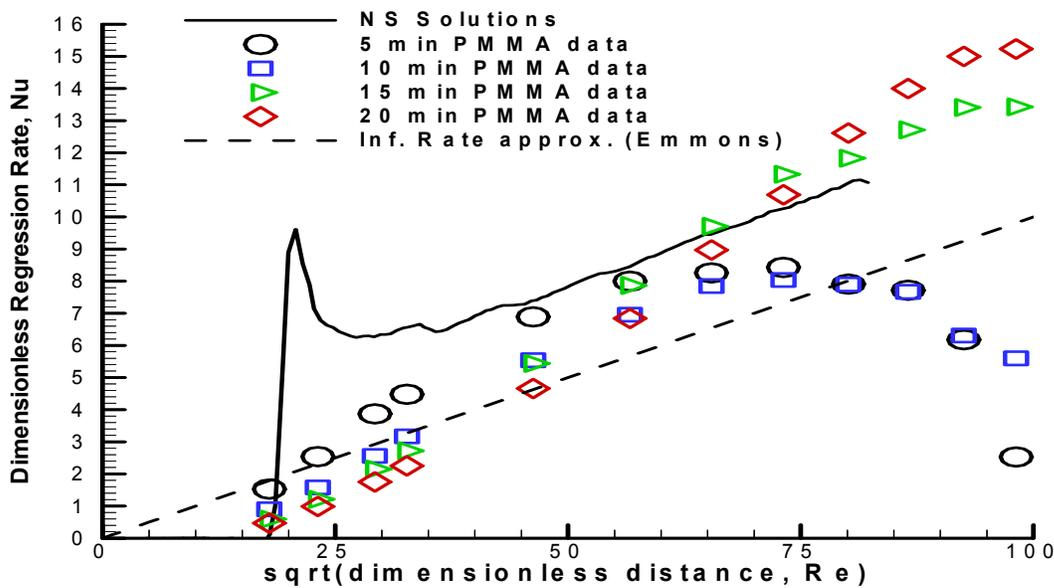
**Figure 6 Comparison of Steady State NS Solutions and BL theory with PMMA Experiments Performed for Different Burn Times and at Fixed  $U=168$  cm/sec**
