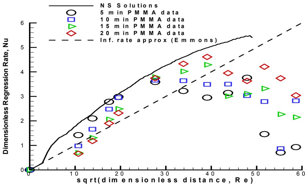
**Figure 3 Comparison of Steady State NS Solutions and BL theory with PMMA Experiments Performed for Different Burn Times and at Fixed  $U = 60$  cm/sec**
