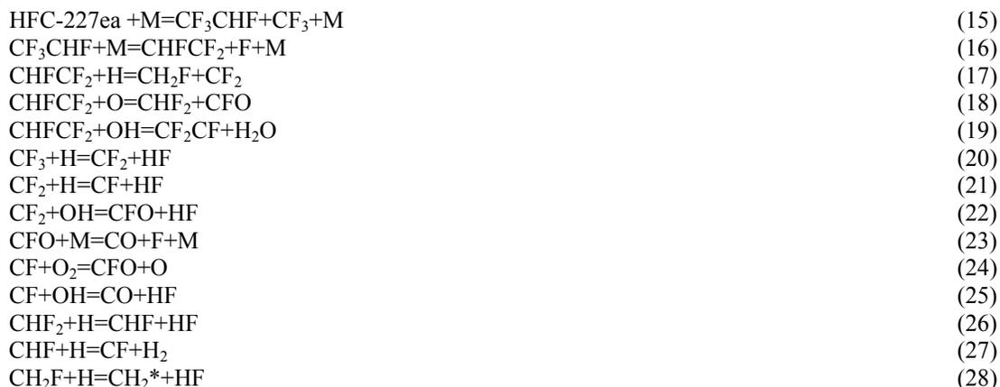
Calculations of different composition ratios of HFC-227ea with NaHCO<sub>3</sub> demonstrated that the main reaction between the two compounds is the formation of NaF, which is caused by the reaction of sodium atom with CF<sub>2</sub>O in the flame reaction zone as
