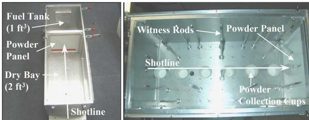
Figure 1. Experimental Test Device and Powder Collection Methods
