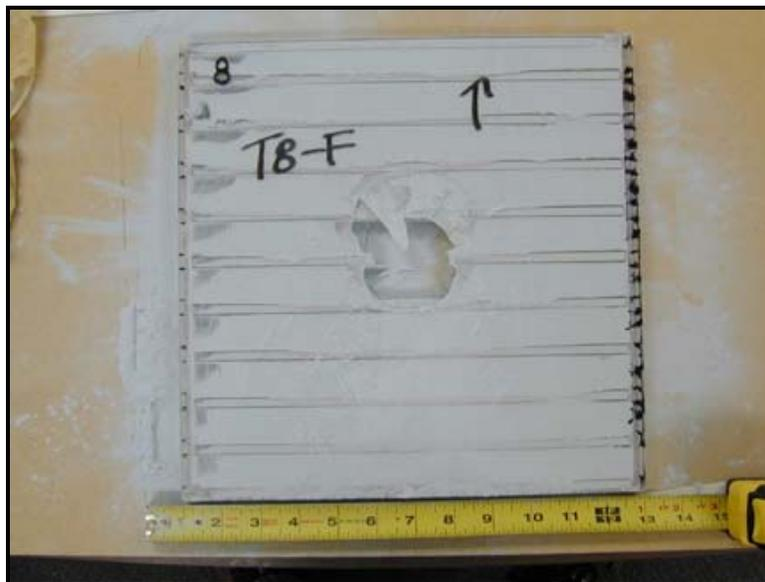
Figure 3. Rib Design Featuring Hollow Acrylic Tube Channels (Post-Test)
