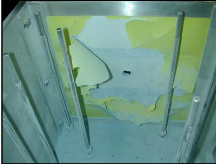
Figure 4. Test Example of Significant Panel Fracture and Material Loss
