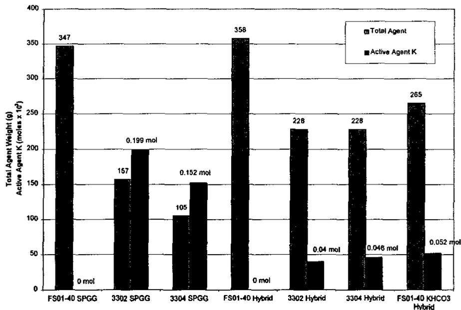
Figure 5. Total agent weight needed to extinguish fire.
