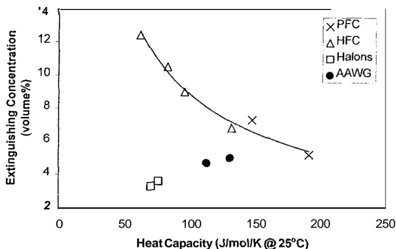
Figure 9. Extinguishing concentration vs. heat capacity
