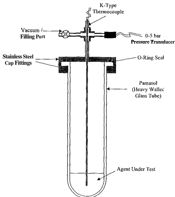
Figure 1. Apparatus for vapour pressure versus temperature measurements.
