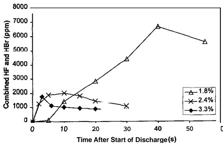
Figure 5. HF concentrations generated during fire tests with BTP (7.3 kWm<sup>-3</sup> heptane fire in 200 L chamber).
