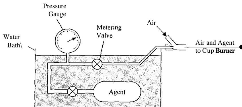
Figure 3. Apparatus for the delivery of low volatility agents into the cup burner.
