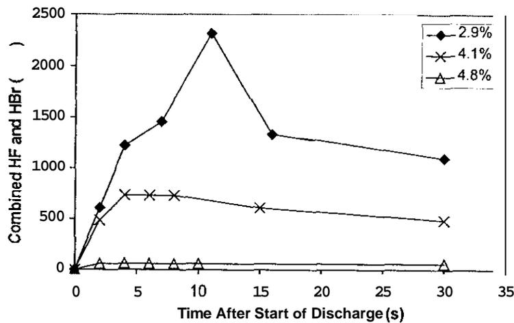
Figure 7. HF concentrations generated during fire tests with Halon 1301 ( $7.3 \text{ kWm}^{-3}$  heptane fire in 200 L chamber).
