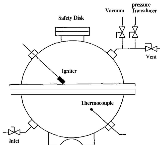
Figure 8. Apparatus for inerting measurements.
