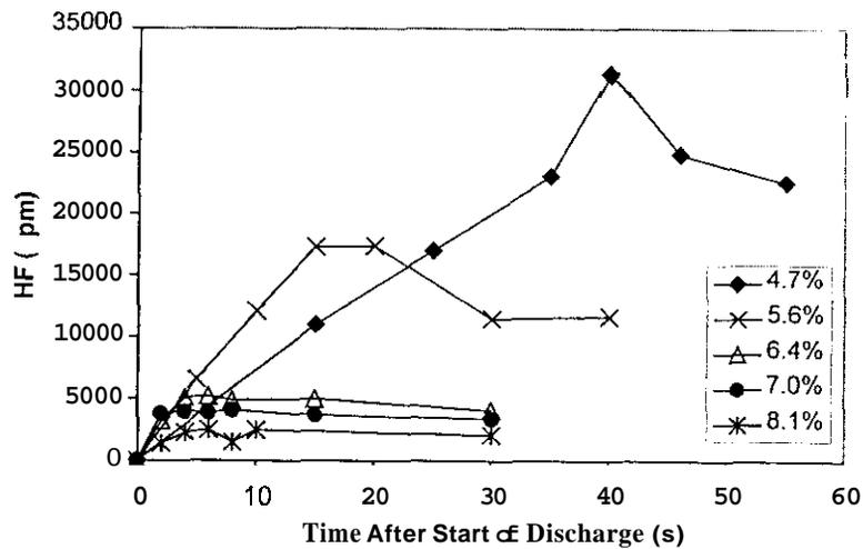
Figure 6. HF concentrations generated during fire tests with HFC-227ea ( $7.3 \text{ kWm}^{-3}$  heptane fire in 200 L chamber).
