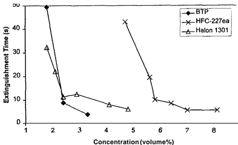
Figure 4. Comparison of the extinguishing efficiencies of BTP, HFC-227ea, and Halon 1301.
