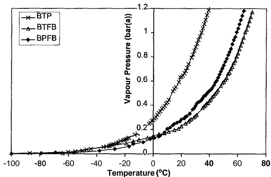
Figure 2. Dependence of the vapour pressure on temperature for the three agents tested.
