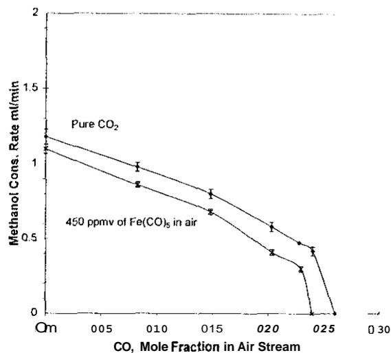
Figure 2. Methanol consumption rate in cup-burner flame as a function of added CO, mole fraction with and without 450 ppm  $\text{Fe}(\text{CO})_5$  added to the air stream.
