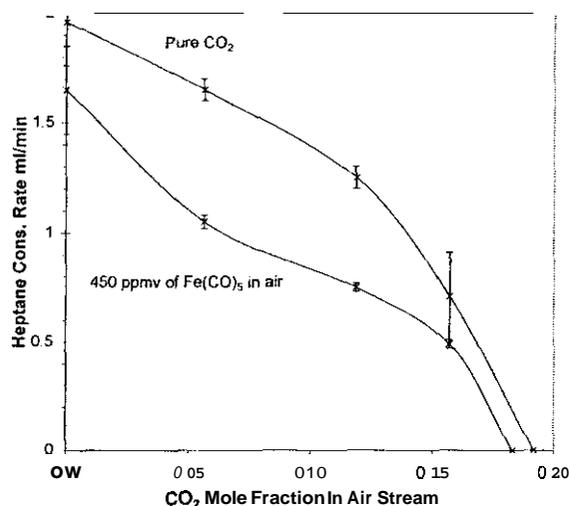
Figure 1. Heptane consumption rate in cup-burner flame as a function of added CO, mole fraction with and without 450 ppm  $\text{Fe}(\text{CO})_5$  added to the air stream.
