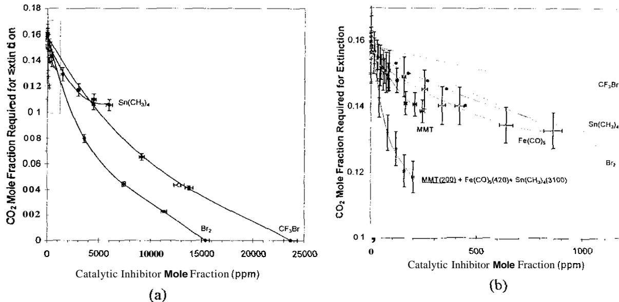
Figure 3. Mole fraction of CO<sub>2</sub> required for methane-air cup-burner flame extinction as a function of catalytic inhibitor mole fraction, CF<sub>3</sub>Br, Br<sub>2</sub>, Fe(CO)<sub>5</sub>, TMT, MMT, or a blend of the last three (b. has expanded x- and y-axes compared to a.).
