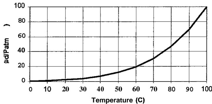
Figure 2. Saturation pressure of water in air at atmospheric pressure.
