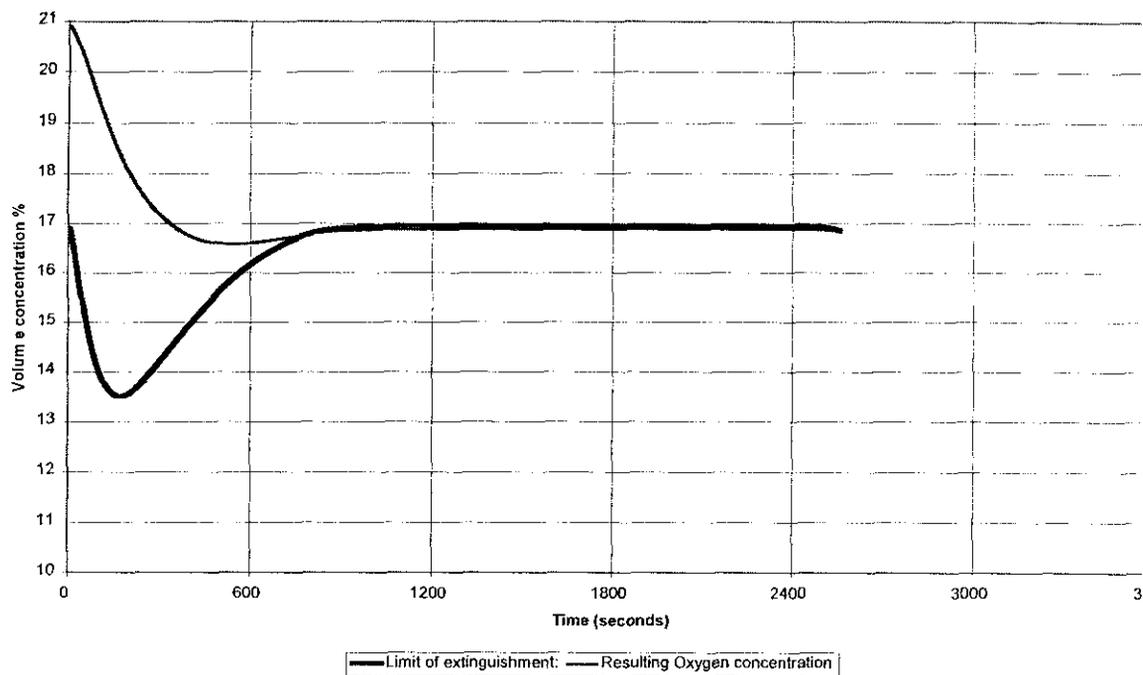
Figure 8. Oxygen concentration and extinguishment limit in a 3000 m<sup>3</sup> enclosure, 3 m<sup>2</sup> pool fire.
