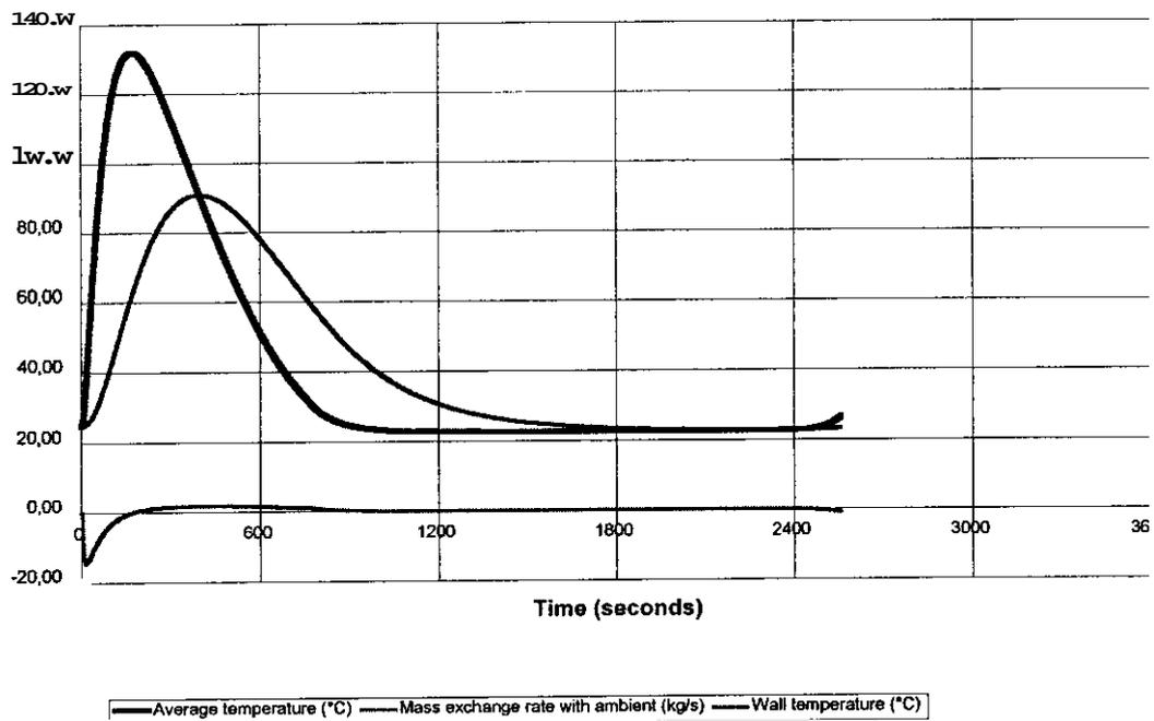
Figure 7. Temperatures and mass exchange rate in a 3000 m<sup>3</sup> enclosure, 3 m<sup>2</sup> pool fire.
