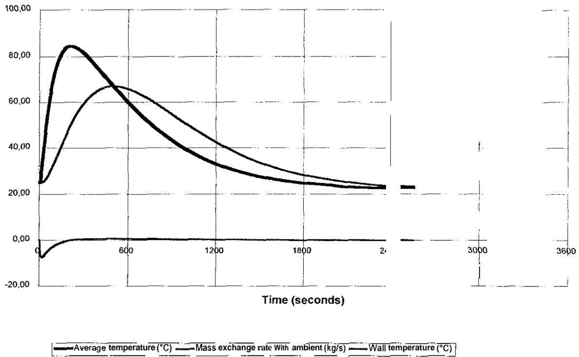
Figure 4. Temperatures and mass exchange rate in a 3000 in' enclosure, 1.5 m<sup>2</sup> pool fire
