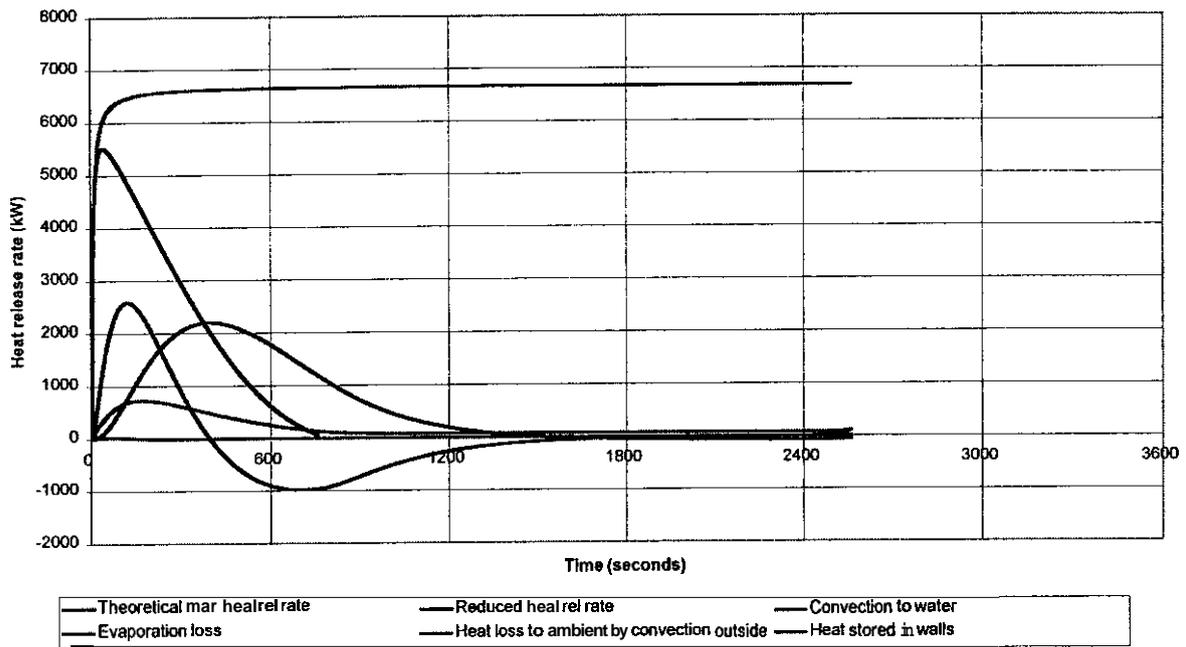
Figure 6. Heat balance of compartment and heat release rate of fire, in a 3000 m<sup>3</sup> enclosure, 3 m<sup>2</sup> pool fire.
