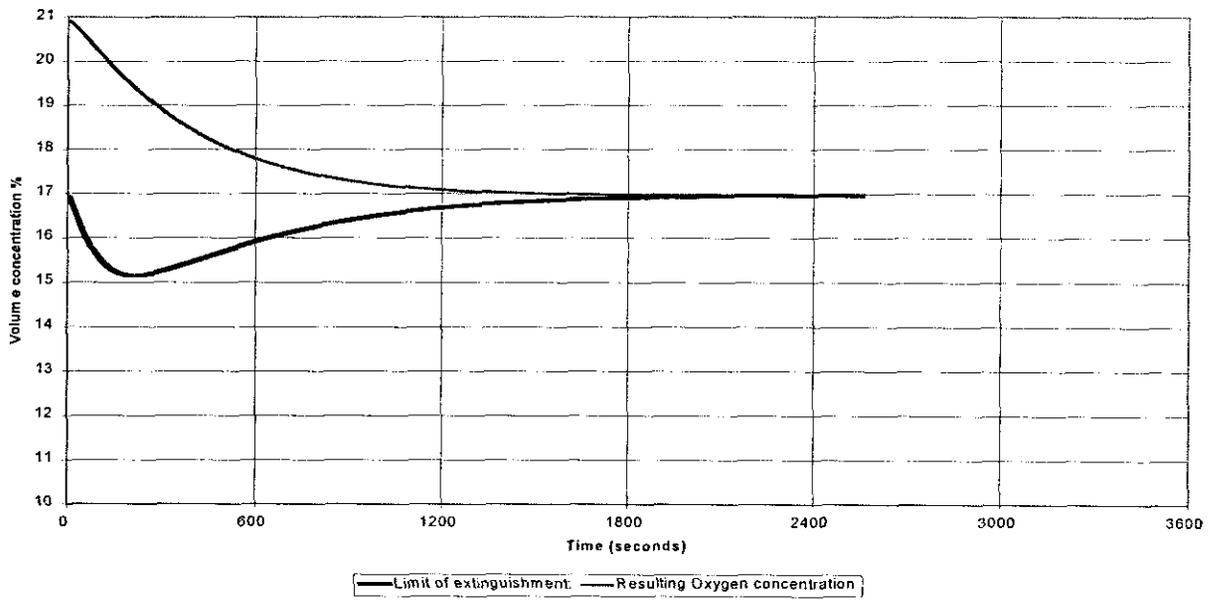
Figure 5. Oxygen concentration and extinguishment limit in a 3000 m<sup>3</sup> enclosure, 1.5 m<sup>2</sup> pool fire.
