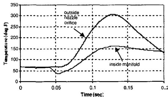
Figure 8. FM200 hybrid exhaust temps.
