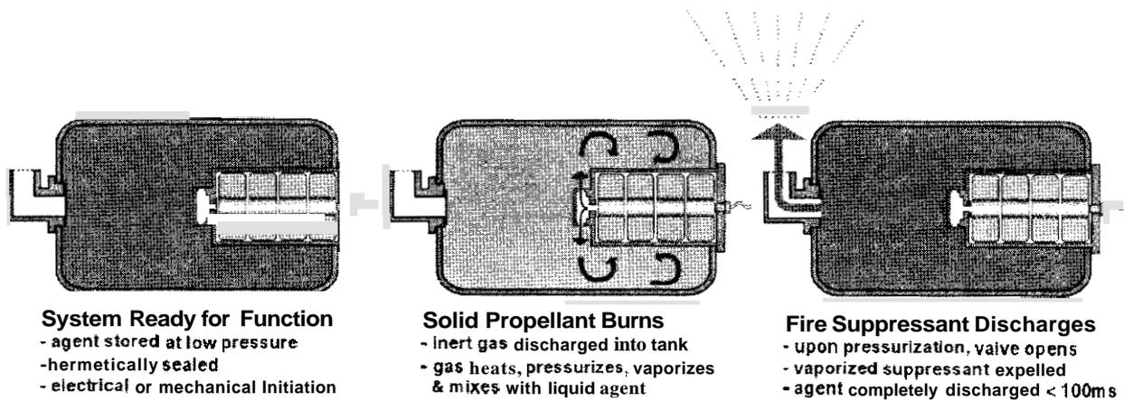
Figure 3. Schematic of a hybrid fire extinguisher discharge process.
