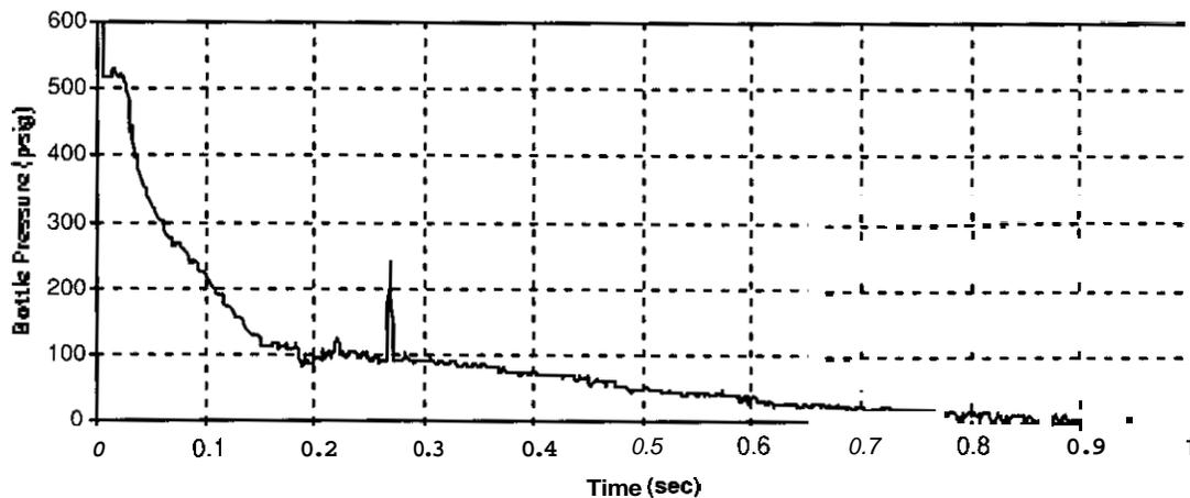
Figure 14. FM200 Blow-down system bottle pressure after  $-40^{\circ}\text{C}$  soak.
