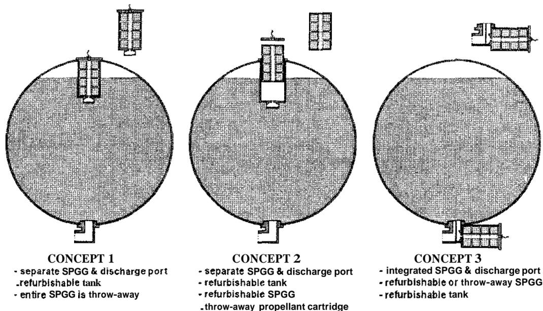
Figure 6. Three functionally equivalent hybrid fire extinguisher configurations.
