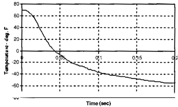
Figure 12. FM200 blow-down system exhaust temperature.
