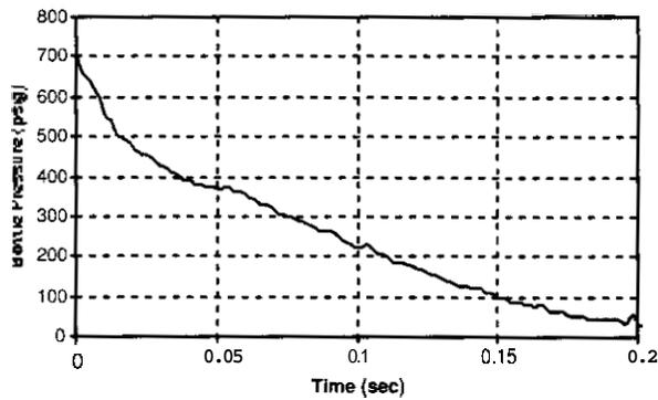
Figure 11. FM200 blow-down system bottle pressure.
