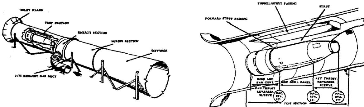
Figure 4. FAA Engine Nacelle Test Facility. Figure 5. Power plant installed in wind tunnel.
