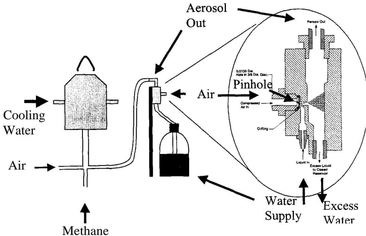
Figure 1. Schematic of experimental configuration. Enlarged image is from TSI Instruction manual, Part Number 133076 – Rev. F (used with permission).
