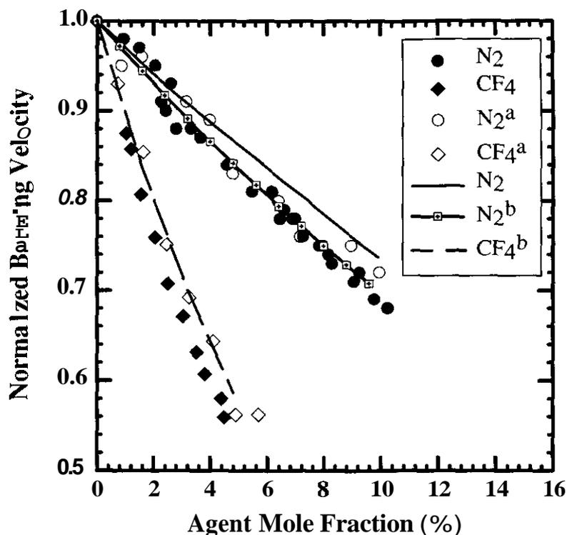
Figure 2. Premixed methane-air burning velocity as a function of agent mole fraction, normalized by the uninhibited burning velocity. Closed points represent measurements from present study, open points (a) are from [1]. Solid line shows calculations from the present study using PREMIX with GRI-Mech. Dashed line and line with square/cross (b) are from [4].
