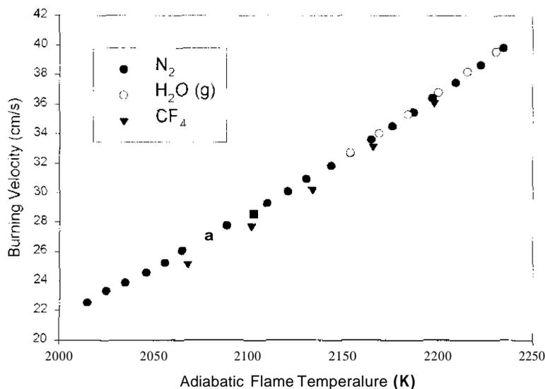
Figure 3. PREMIX calculations of burning velocities of stoichiometric methane/air mixtures inhibited by various concentrations of nitrogen,  $\text{CF}_4$ , and water vapor, plotted as a function of the adiabatic flame temperature.
