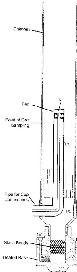
Figure 2. Technical drawing of the cup burner
