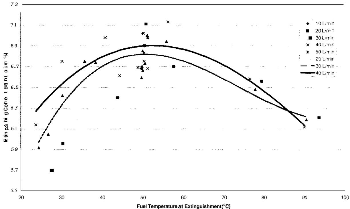
Figure 4. Variation of HFC-227ea extinguishing concentration with fuel temperature.
