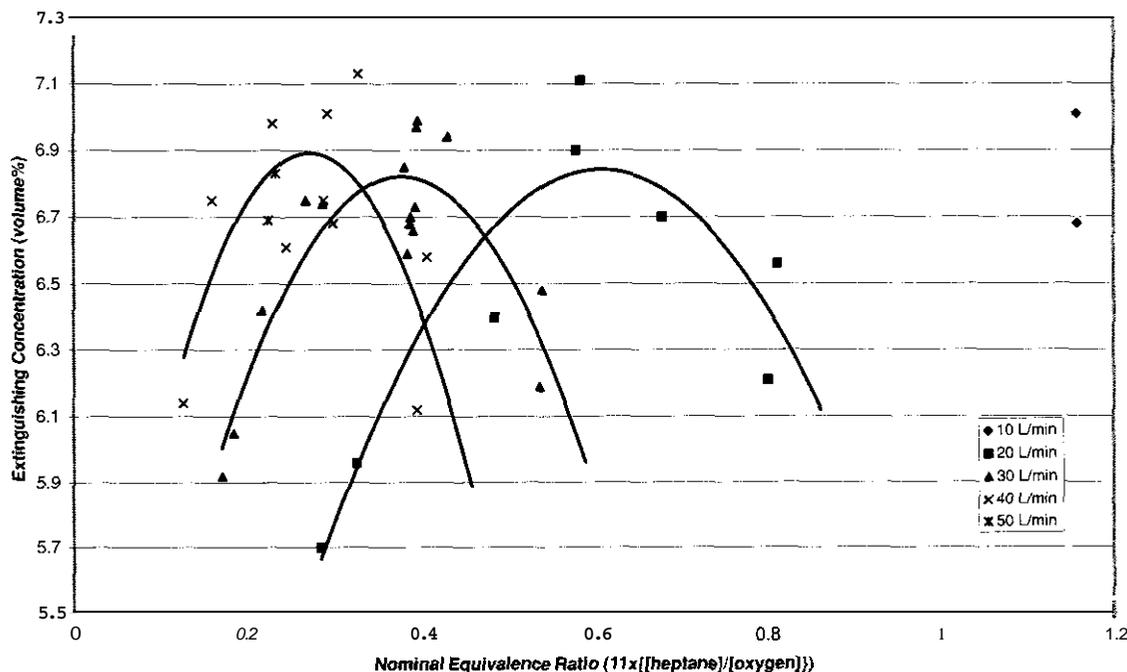
Figure 8. Variation of HFC-227ea extinguishing concentration with nominal equivalence ratio.
