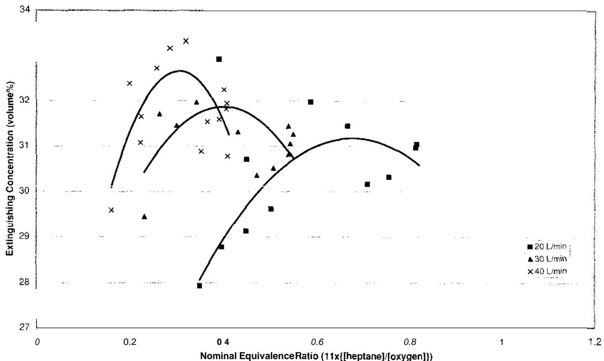
Figure 9. Variation of nitrogen extinguishing concentration with nominal equivalence ratio.
