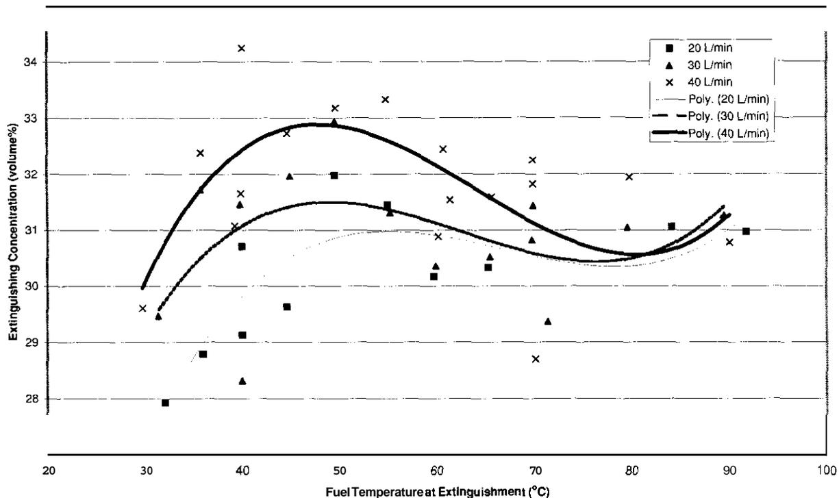
Figure 5. Variation of nitrogen extinguishing concentration with fuel temperature.
