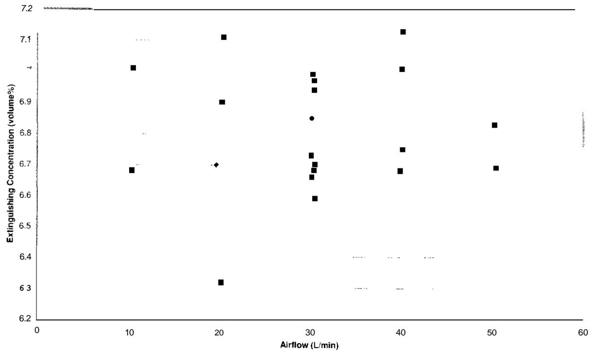
Figure 6. Dependence of the HFC-227ea extinguishing concentration on air flow.
