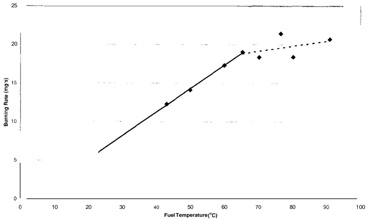
Figure 7. Dependence of the n-heptane free burning rate on temperature.
