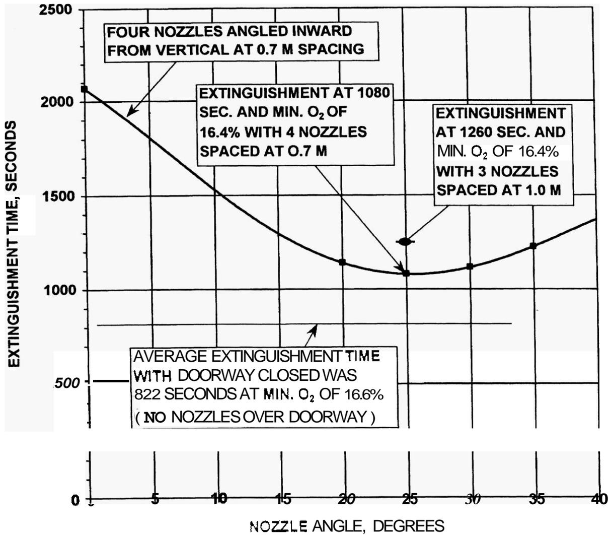
EXTINGUISHMENT TIME VERSUS ANGLE OF 4 M<sup>2</sup> DOORWAY SCREENING NOZZLES FOR 1.1 MW LOW PRESSURE/LOW FLOW CONCEALED DIESEL OIL SCENARIO 6 FIRE TESTS WITH AM4 *AquaMist* NOZZLES OPERATING AT 12.8 BAR IN 1280 M<sup>3</sup> ENCLOSURE AND NOZZLE DIFFUSERS 0.2 M BELOW THE CEILING
