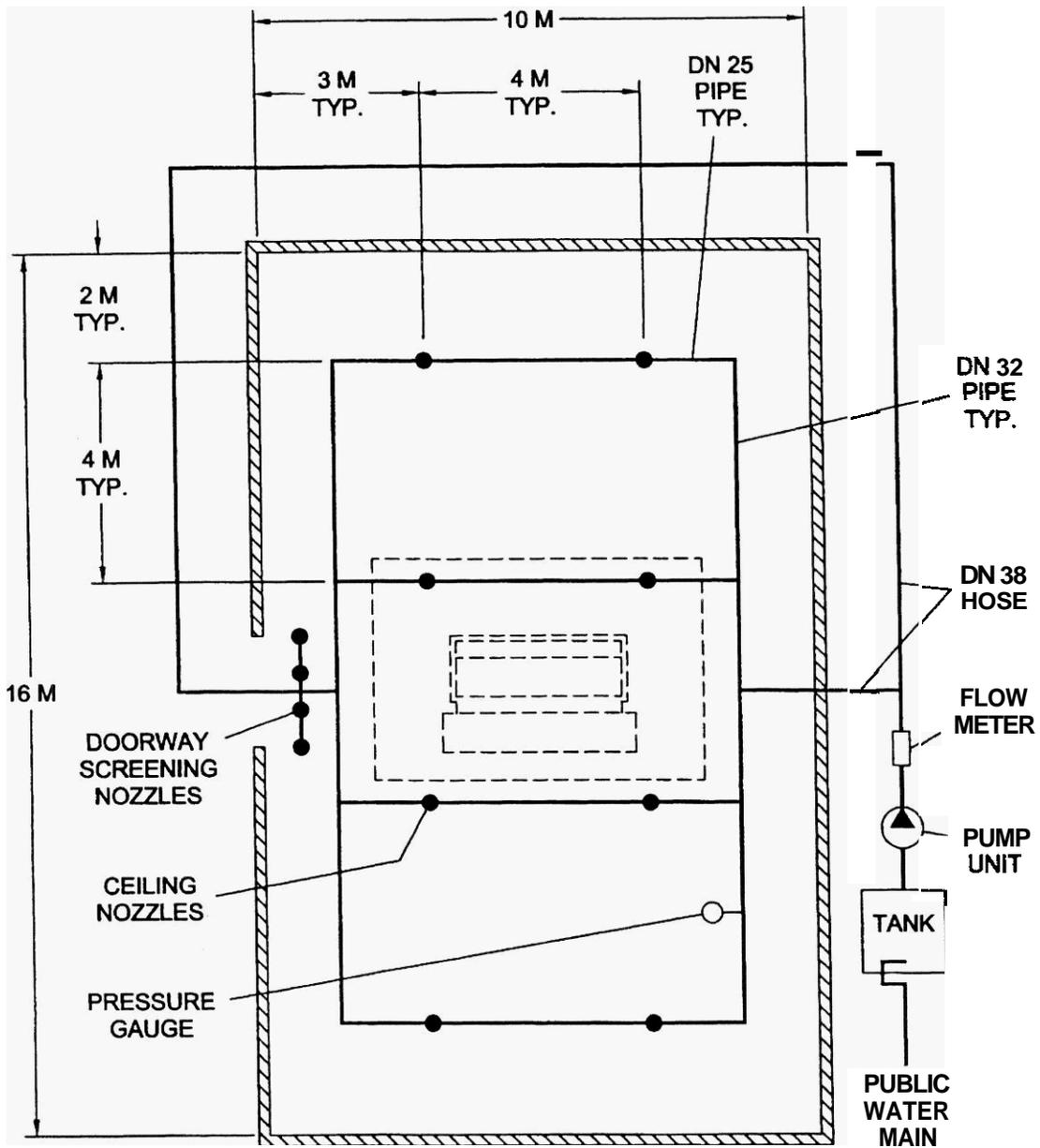
PLAN VIEW LAYOUT OF ENCLOSURES AND PIPING USED FOR TESTING OF AM4 NOZZLES IN THE 800 M<sup>3</sup> AND 1200 M<sup>3</sup> EVALUATIONS
