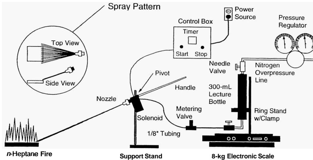
Figure 1. Laboratory-Scale Apparatus for screening of Candidate Streaming Agents.
