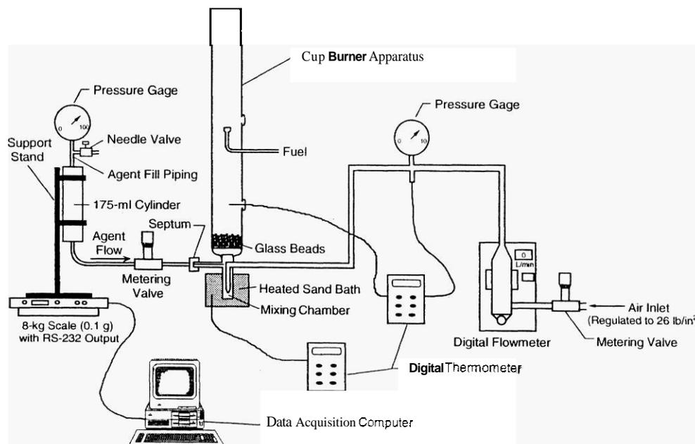
Figure 2. Cup-Burner Schematic.
