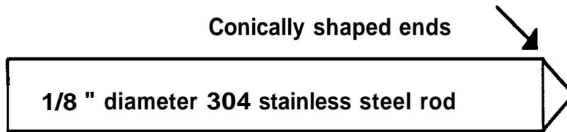
Figure 3. Conical Type Electrode.
