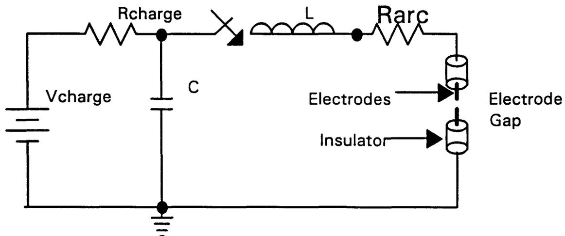
Figure 5. Typical Discharge Circuit.
