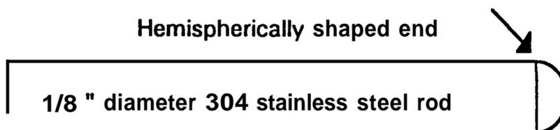
Figure 2. Hemispherical Type Electrode.
