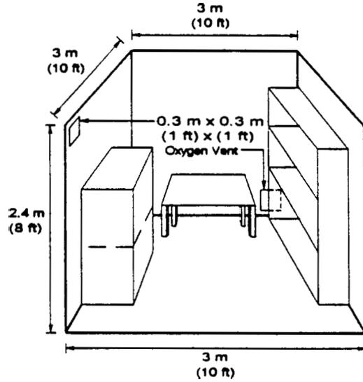
Fig. 1 - Simulated flammable liquid storeroom
