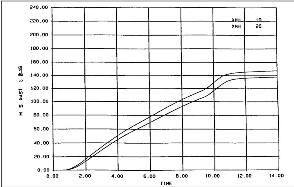
**Predicted Integrated Mass Flow from Two of Nine Nozzles**
