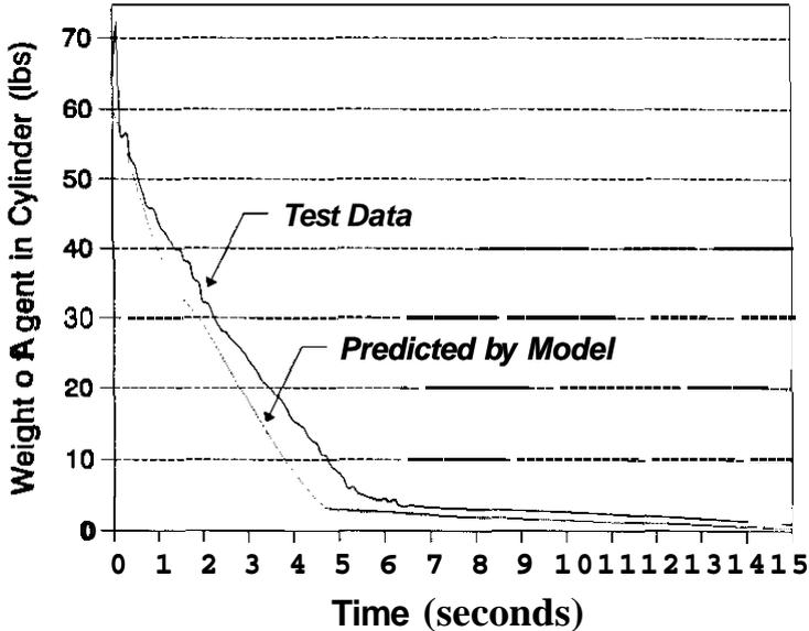
**Figure 5:** Comparison of Measured and Predicted Weights of Agent in Cylinder for Test 4 (HFC-227ea)
