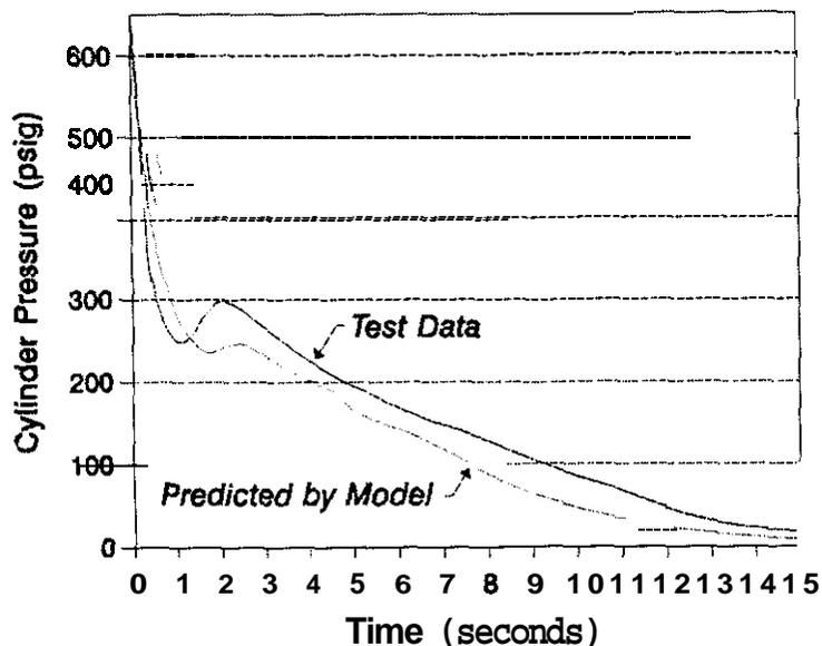
Figure 4 Comparison of Measured and Predicted Cylinder Pressures for *Test 4* (HFC-227ea)
