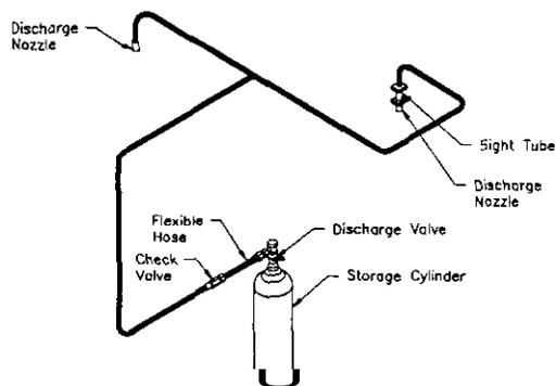
Figure 2: Double Nozzle Discharge System
