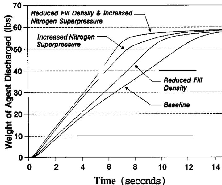
Figure 7: Predicted Discharge Characteristics for Alternate Fill Densities and Storage Pressures (HFC-227ea)
