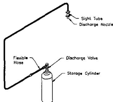
Figure 1: Single Nozzle Discharge System
