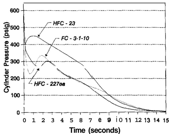
Figure 3: Cylinder Pressure During Discharge of HFC-23 (Test 7), FC-3-1-10 (Test 11), and HFC-227ea (Test 2)
