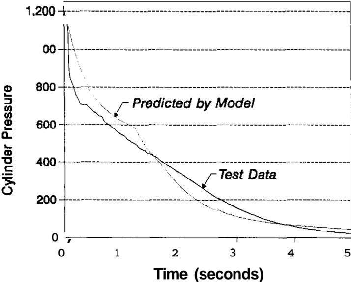
**Figure 6:** Comparison of Measured and Predicted Cylinder Pressures for Test 13 (HFC-227ea)
