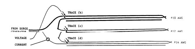
Figure 1. Series connection of test cables
