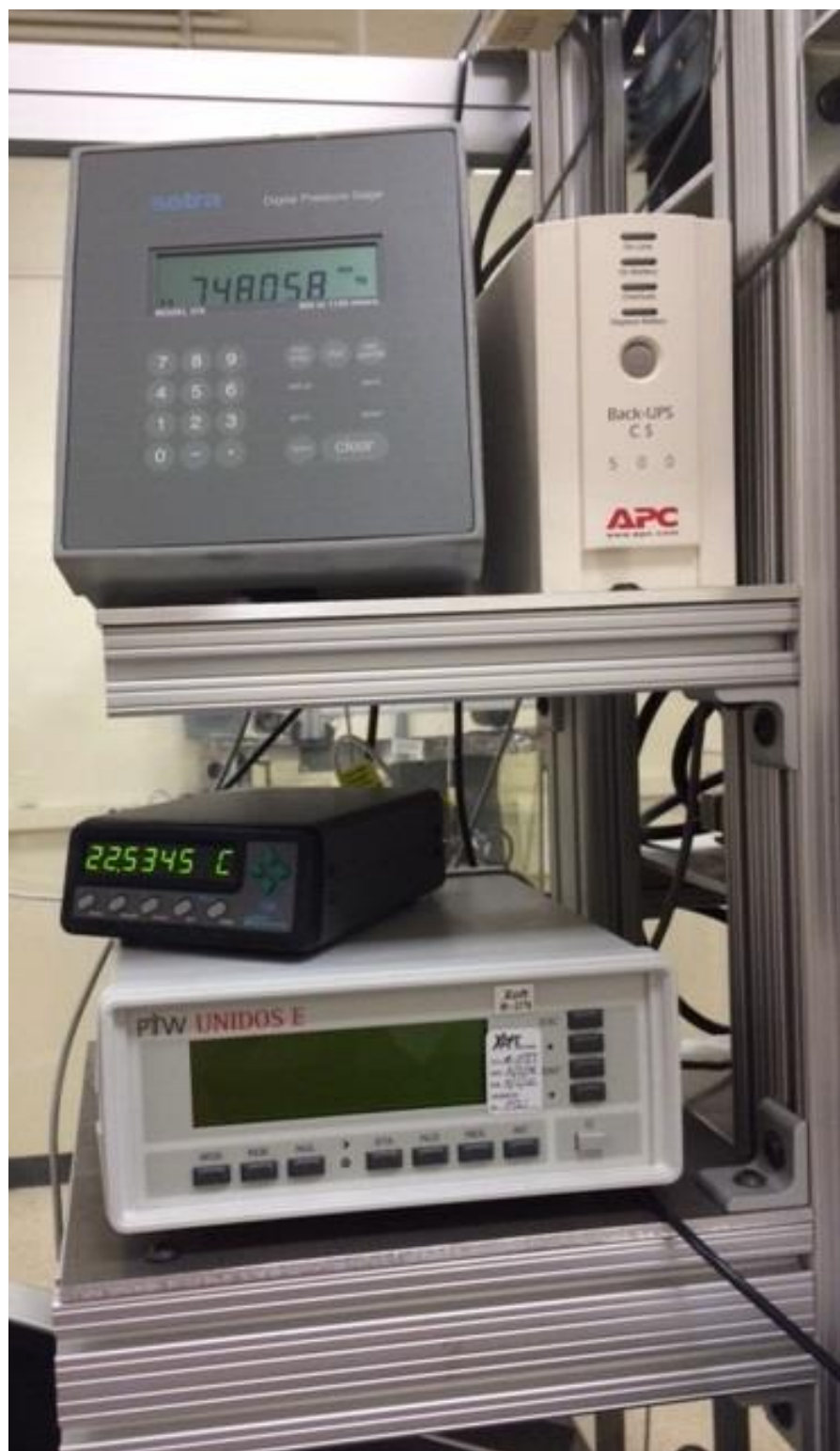
Figure 7. Barometer, thermometer and well-chamber electrometer.
