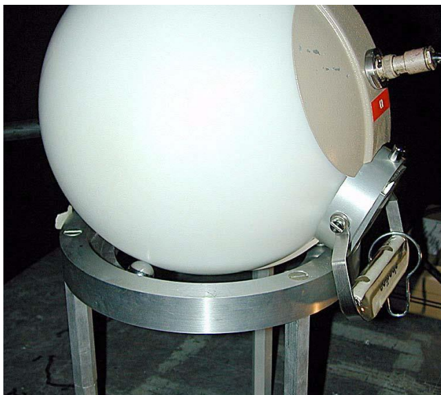
Figure 3: Mechanical design of the rem ball ring stand.
