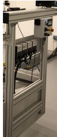
Telescope stand with motion control and EMO
