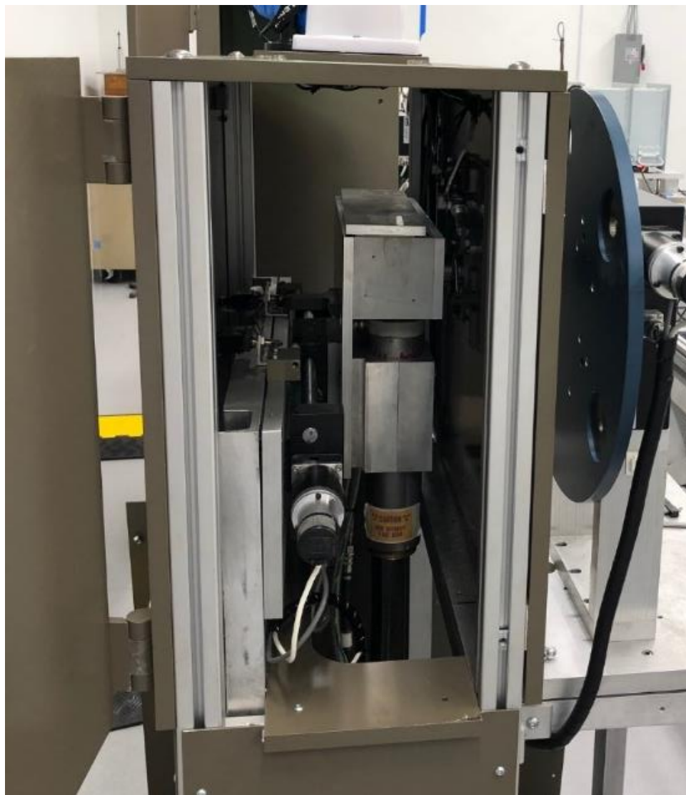
Figure 10 The mammography translation tube support.
