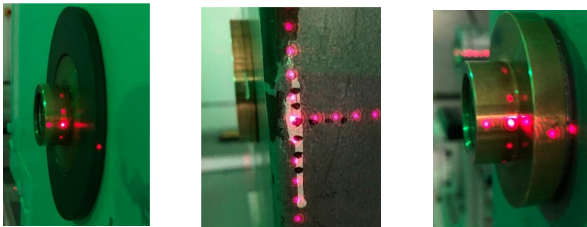
Figure 19 Alignment points of standards, showing laser crosshair.
