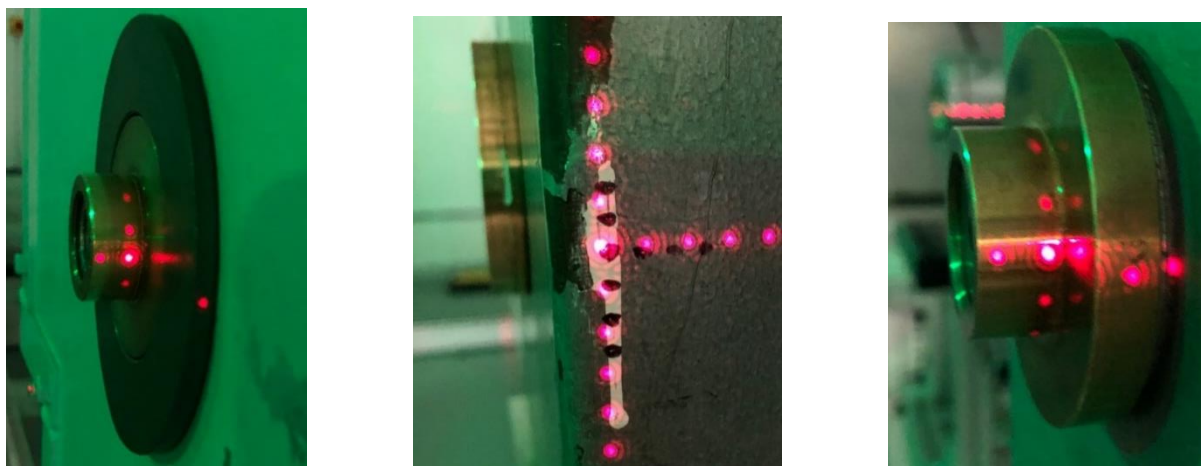
Figure 19 Alignment points of standards, showing laser crosshair.
