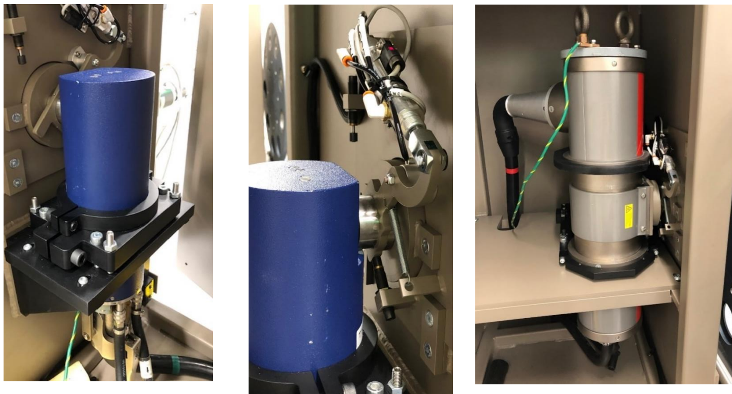
Figure 11 The 100 kV tube and closeup of the shutter assembly on left and center picture and the 300 kV tube shown in the right picture.
