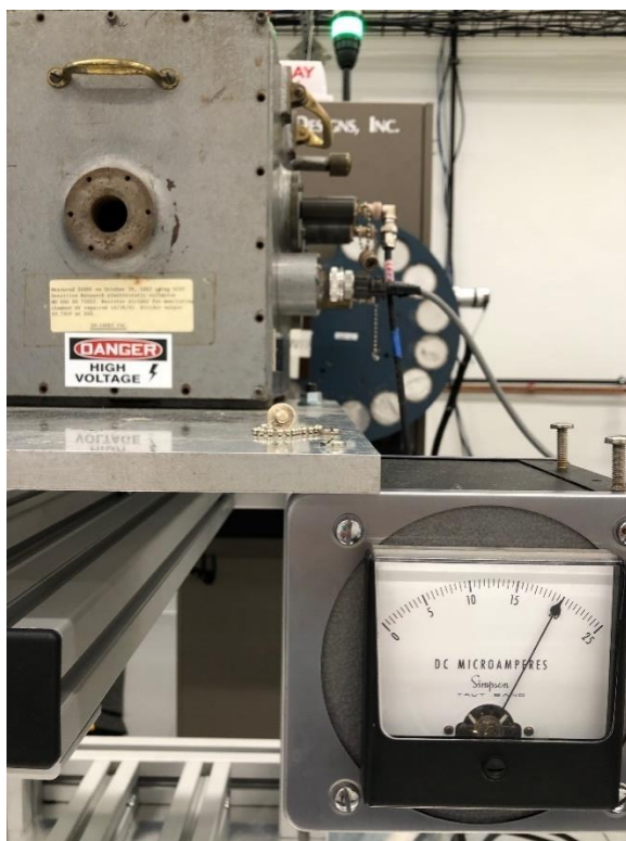
Figure 20 The Ritz (left) and Wyckoff-Attix (right) chamber meters showing voltage application.
