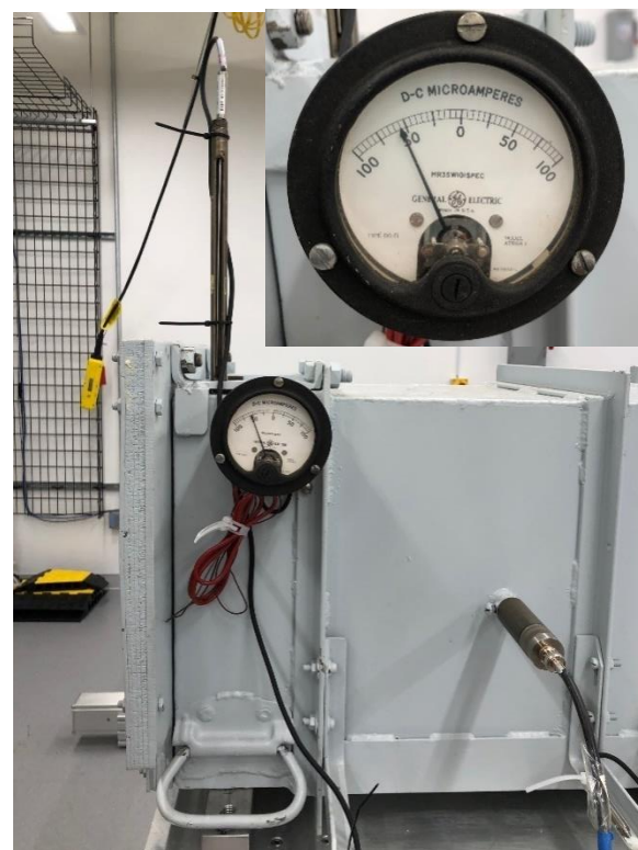
Figure 20 The Ritz (left) and Wyckoff-Attix (right) chamber meters showing voltage application.
