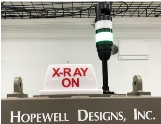
Calibrator "x-ray on" light illuminates when the generator is energized
