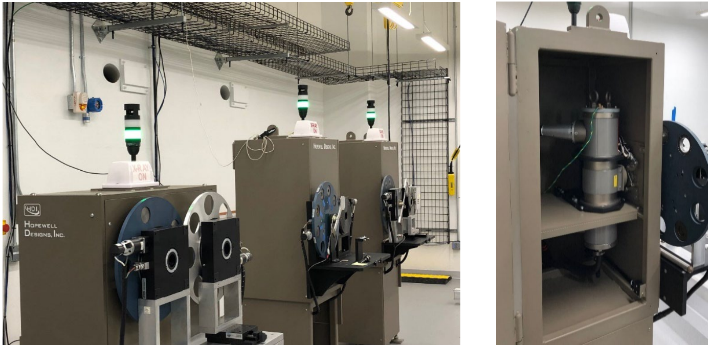
Figure 9 The three x-ray calibrators, showing the interior of the 300 kV calibrator with x-ray tube.
