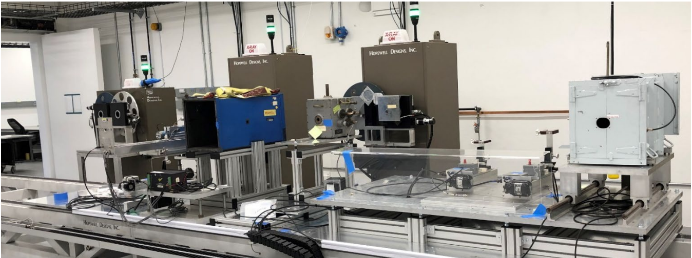
Figure 2b Position of the device under test (DUT) from right to left: 300 kV FAC, T1, T2, 100 kV FAC, Mammo FAC, T3 and T4 .
