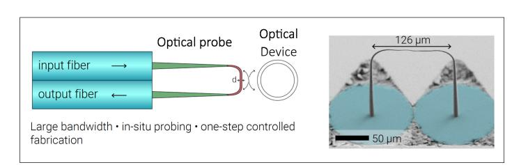
The TPOP optical probe provides highly local probing of PICs, including optical devices and light sources located on-chip for developing next generation technologies.
