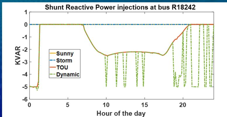
Figure MIT-12 Shunt capacitor reactive power injections at node 'R18242'
