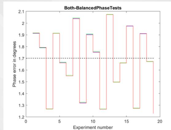
Line compensated Phase difference computed using a 5E4 sample DFT – Phase steps [0:  $\pi$ ] rad
