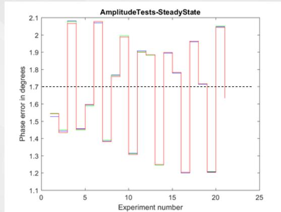
Line compensated Phase difference computed using a 5E4 sample DFT – Amplitude steps [1: 0.3: 7]  $V_{rms}$
