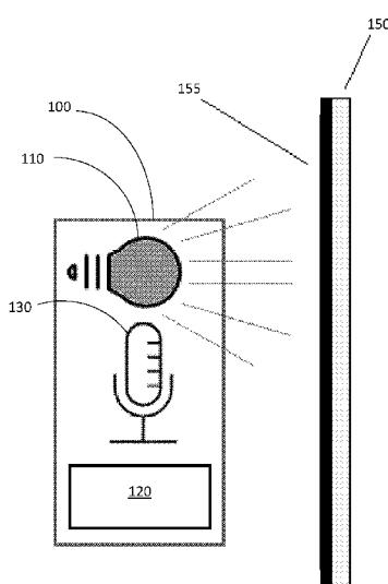
(57) Abstract: An apparatus and method for measuring soot deposition includes irradiating a soot deposit with pulsed electromagnetic radiation configured to cause a rapid-enough expansion of the soot deposit to cause an acoustic pressure wave, sensing the pressure wave with an acoustic measurement device, and, based on the received signal and calibration data, determining the amount of soot deposited.
