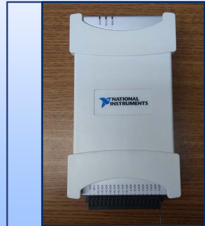
Data Acquisition Device
