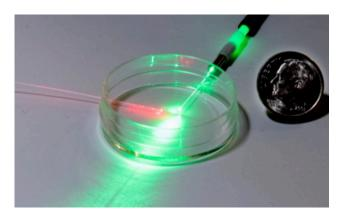
An empty petri dish with two optical fibers, illustrating one version of the researchers' experiment. The left-hand fiber (usually shining infrared light, but depicted here as visible red light) is a temperature sensor. The top fiber shines green, red or blue light into the petri dish to adjust the signal that the temperature sensor measures.
