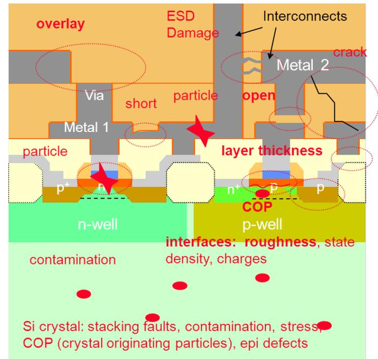
*Examples of yield distracting defects possible during microelectronics production processes (source: ITRS YE chapter)*
