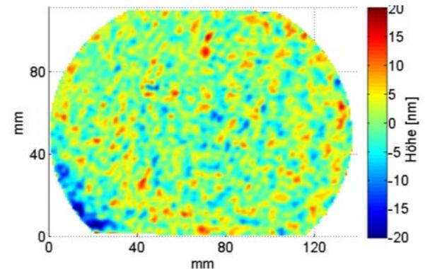
Flatness (top) and Nanotopography (bottom) of a polished Si wafer
