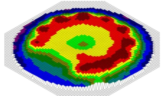
Film thickness map of a 2 nm SiON film with 9% nitrogen
