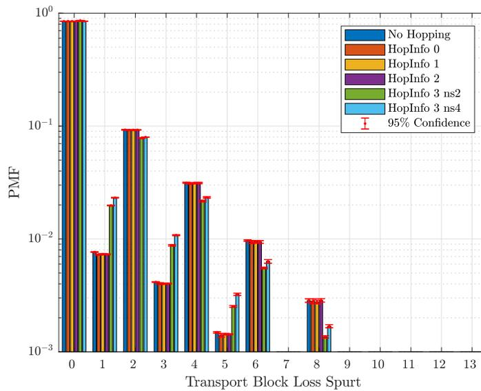
**Fig. 20.** Transport block loss spurt for D2D communication group size 100, MCS 10,  $K_{TRP} = 2$ .
