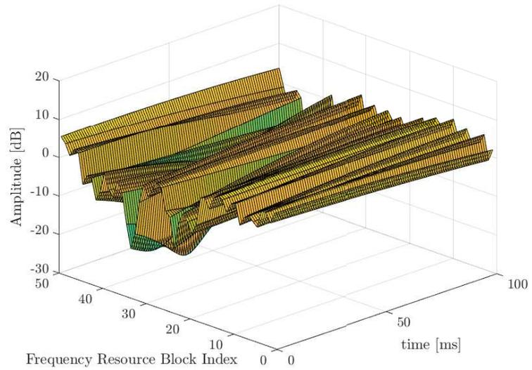
**Fig. 9.** Fading trace sample using Extended Typical Urban model (ETU), LTE band 14, and 3 km/h speed.
