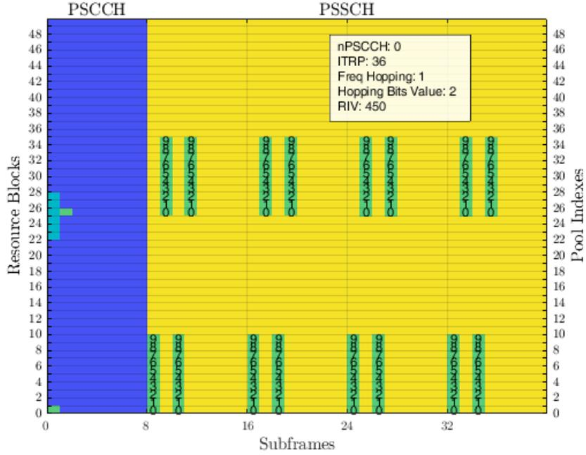
**Fig. 5.** Example sidelink communication resource scheduling for 10 RBs with frequency hopping Type 1, hopping information bits = 2 (decimal representation).
