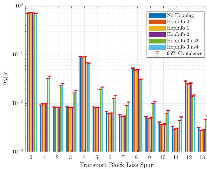
**Fig. 21.** Transport block loss spurt for D2D communication group size 100, MCS 6,  $K_{TRP} = 4$ .
