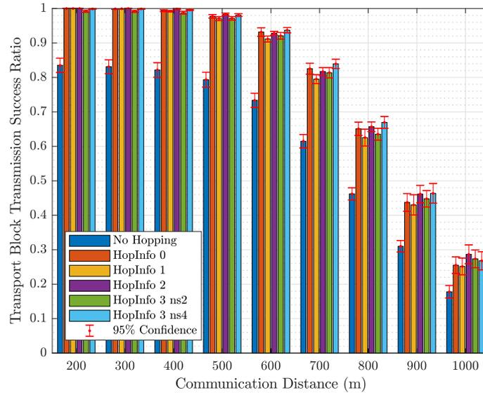
**Fig. 14.** Transport block success rate for single sidelink, MCS 10,  $K_{TRP} 2$ , sidelink period 40 ms, and 10 RBs interference.
