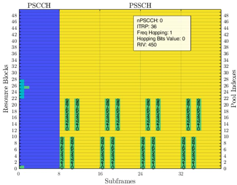
**Fig. 3.** Example sidelink communication resource scheduling for 10 RBs with frequency hopping Type 1, hopping information bits = 0 (decimal representation).
