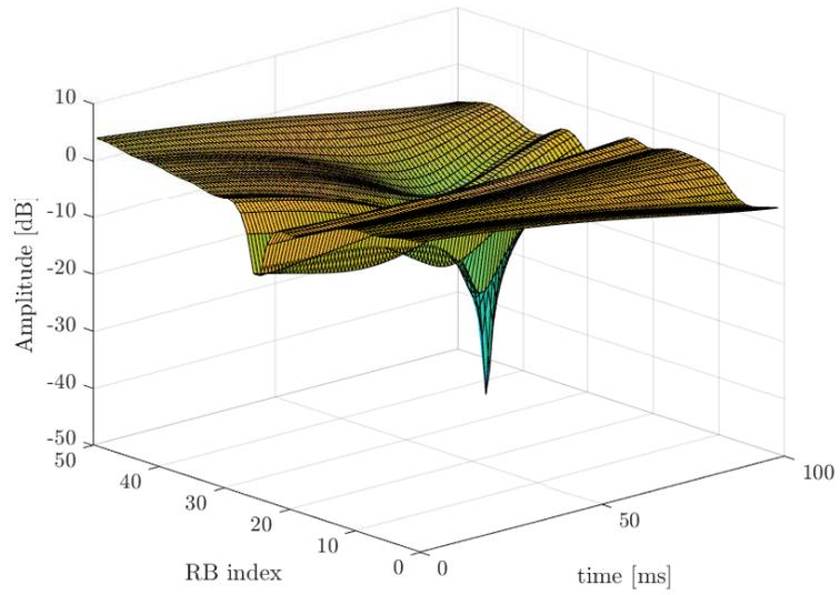
**Fig. 8.** Fading trace sample using Extended Pedestrian A model (EPA), LTE band 14, and 3 km/h speed.
