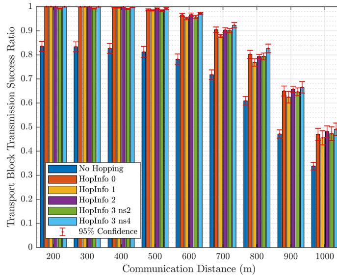
**Fig. 15.** Transport block success rate for single sidelink, MCS 6,  $K_{TRP} 4$ , sidelink period 40 ms, and 10 RBs interference.
