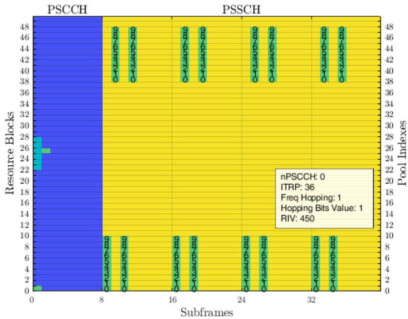
**Fig. 4.** Example sidelink communication resource scheduling for 10 RBs with frequency hopping Type 1, hopping information bits = 1 (decimal representation).
