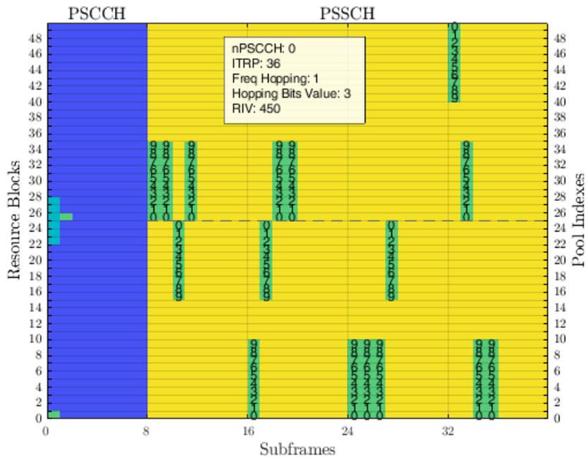
**Fig. 6.** Example sidelink communication resource scheduling for 10 RBs with frequency hopping type 2, and 2 sub-bands.
