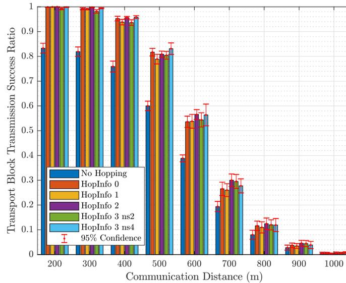
**Fig. 13.** Transport block success rate for single sidelink, MCS 18,  $K_{TRP}$  1, sidelink period 40 ms, and 10 RBs interference.
