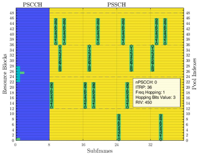
**Fig. 7.** Sidelink communication resource scheduling for 10 RBs with frequency hopping type 2, and 4 sub-bands.
