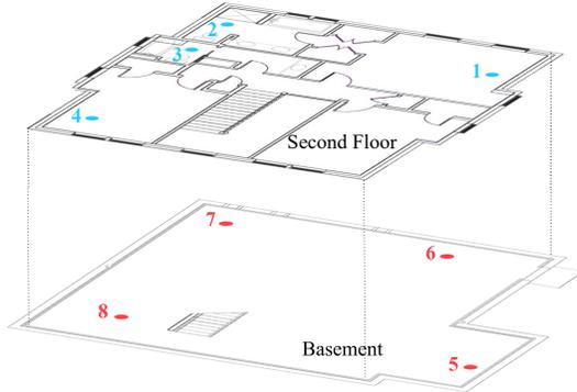
Fig. 6: Radio locations in single-family house extreme tests
