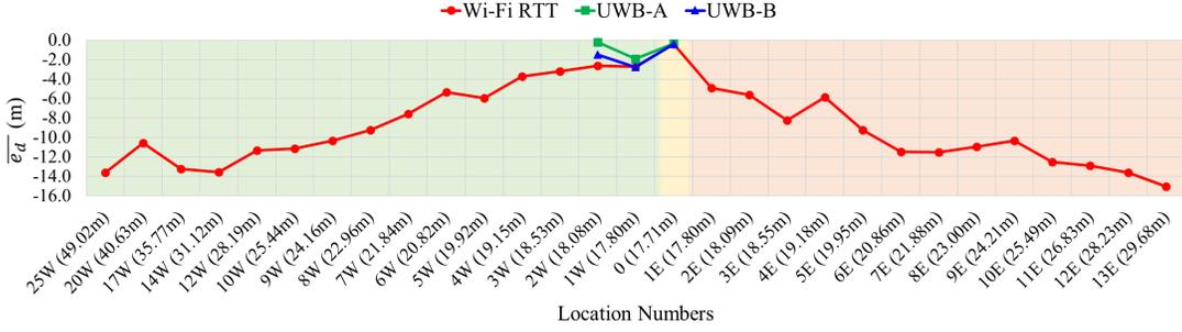
Fig. 14: Average error in the office environment coverage test
