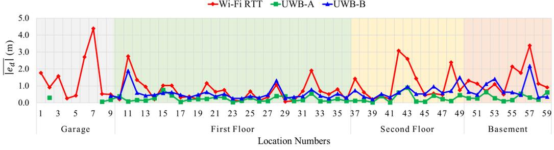
Fig. 15: Mean absolute error in the single-family house coverage test
