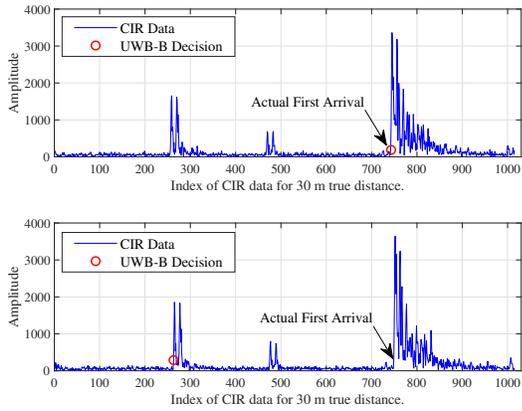
Fig. 10: Two sample UWB-B's CIR sequences
