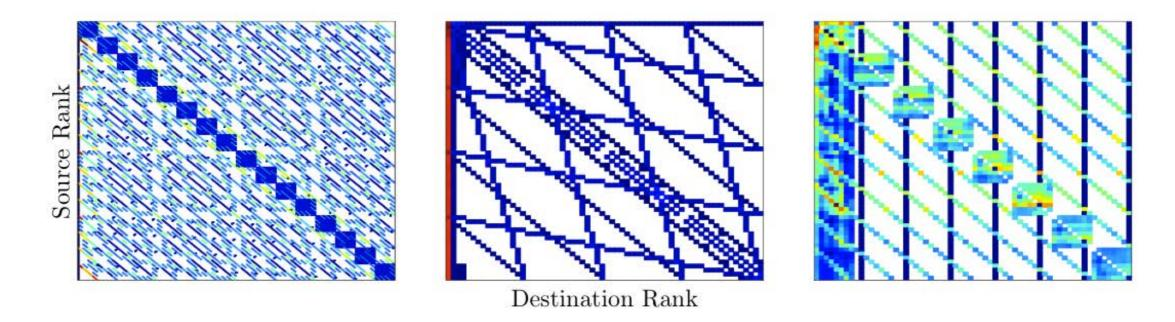
Adjacency matrices for individual runs of a performance benchmark, an atmospheric dynamics simulator, and a linear equation solver SUPERLU (64 nodes).
