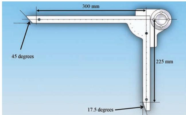
exhibit) and  $Y_1$  to  $Y_{15}$  on the Y axis (vertical in the exhibit). The nominal incremental distance between these target points is 15 mm, which gives a nominal X axis length of 300 mm and nominal Y axis of 225 mm (See Exhibit 8). The X axis is longer because it is intended to approximate the length of an adult femur bone. The distance between any two target holes is measured between the tips of the two holes. Although the
