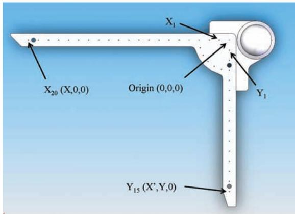
hip acetabulum prosthesis inclination angle. The Y axis bar of the phantom coordinate frame terminates at a nominal 17.5° angle, considered by many as the best choice for the hip acetabulum prosthesis anteversion angle. The femur bar terminates at a nominal 60° angle, preferred by many for decapitation of the damaged head of the femur bone. The arc around the origin of the coordinate XY frame axes has five target holes at nominal
