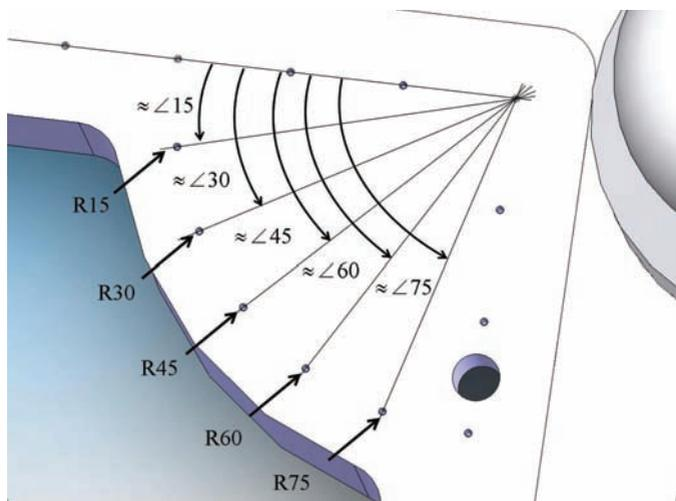
Special attention was given to the drilling of these holes in order to achieve smooth, clean hole walls and tip and hole axis, which is nominally orthogonal to the corresponding coordinate frame XY axes. Several drill bits were used and each was not
