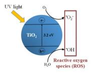
**Figure 1.** Photocatalytic mechanism over TiO<sub>2</sub>. UV light promotes an electron from the valence band (VB) to the conduction band (CB), leaving a hole in the VB and an electron in the CB.
