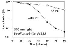
**Figure 3.** Photocatalytic inactivation of *Bacillus subtilis* spores using a cast film of a standard TiO<sub>2</sub>-based photo-catalyst (PC) illuminated with 365 nm light.
