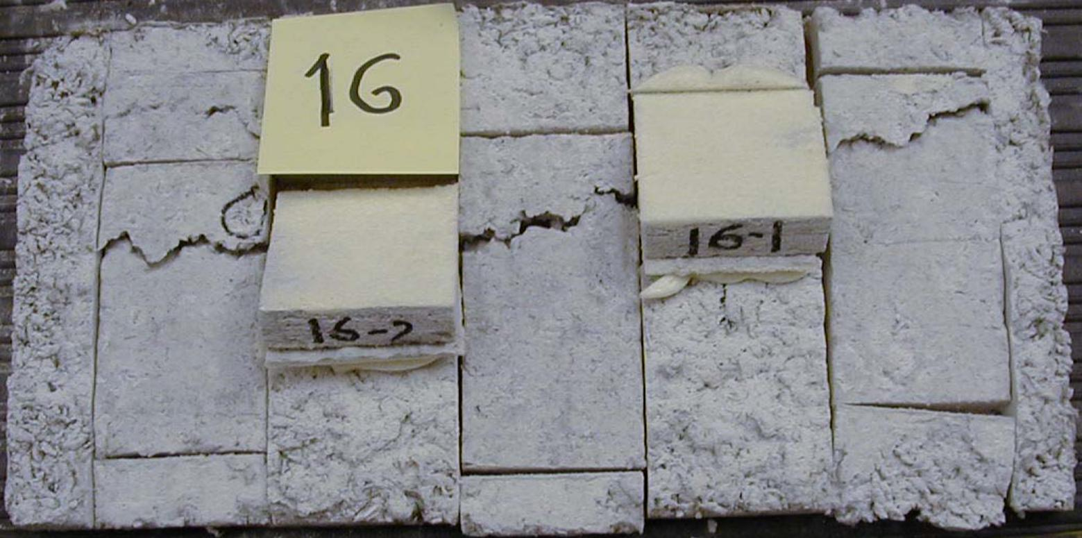
Test 2- Cohesive failure
