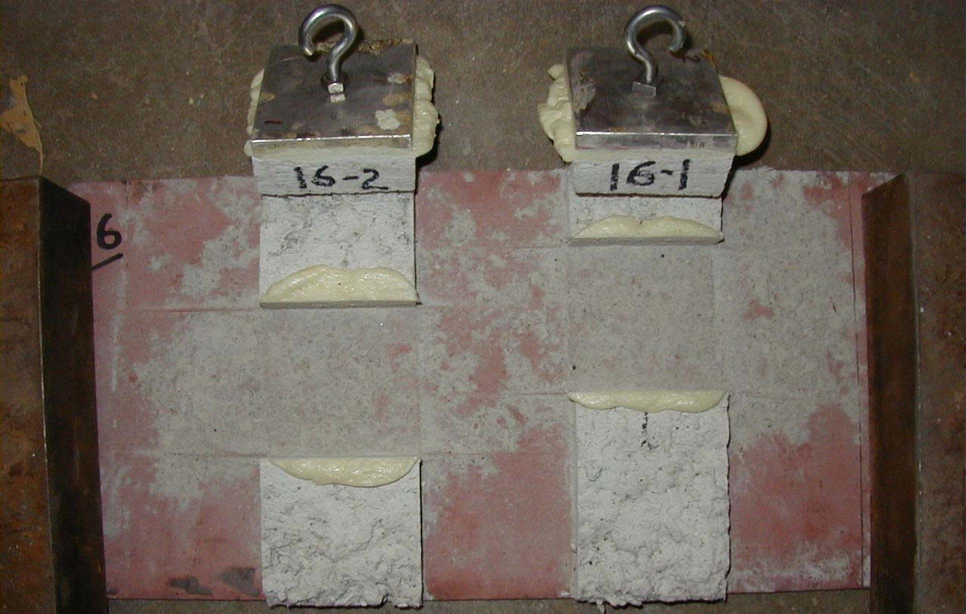
Test 1- Adhesive failure
