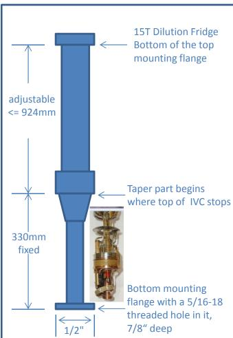
For using with ICEoxford OC/HFBS OC, the distance between the top flange to beam center is 1305mm, plus 4mm Oring =1309mm. With the 15T DR's flange on the very top position, after mounting the cylindrical IVC, the distance between the bottom of the flange and the center of the neutron window is 1310 mm. Perfect fit!
