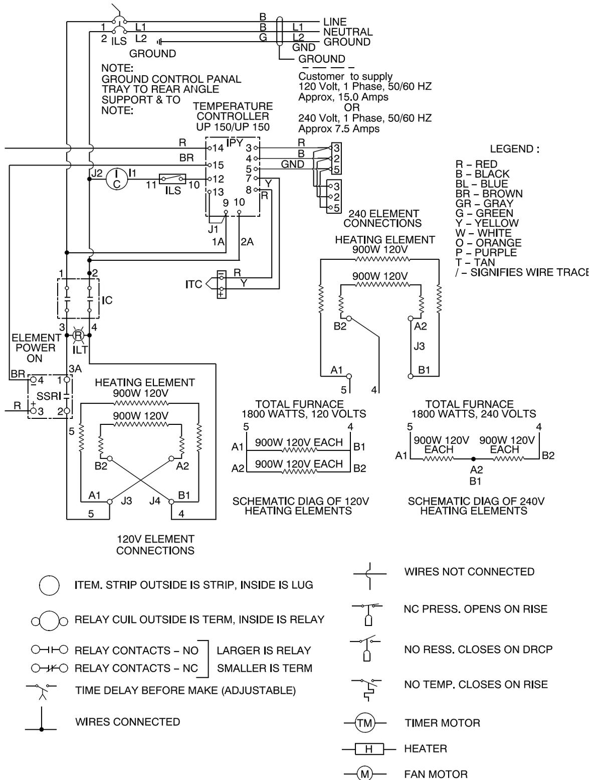
Figure 14. Wiring Diagram (Sheet 2 of 3)
