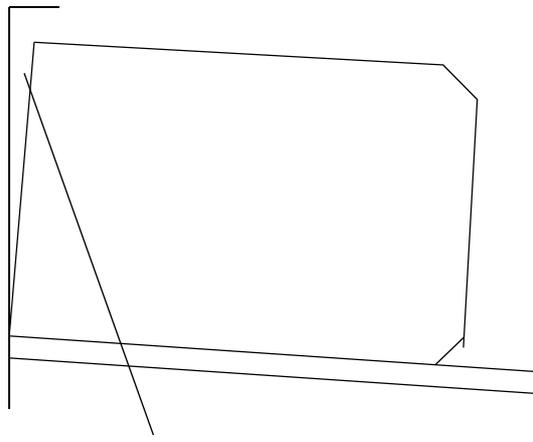
Illustration showing too much gap between top front edge of chamber and front plate of furnace chassis. Adjust platform height with front bottom of chamber flush with front panel of furnace chassis.
