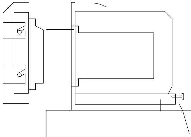
**Figure 13. Alignment of Insulation and Cabinet Front Frame**
