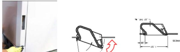
Paper test of the Door insulation seal and EVEN gap between Door and Cabinet.
