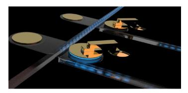
Plasmonic NEMS microdisk enables low loss, high contrast photonic switching with nanosecond response, low voltage and low power dissipation.
