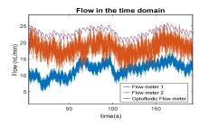
Comparison of NIST flow meter with commercial meters using a 25 nL/min pump (note fine detail of individual motor clicks in the pump mechanism).
