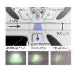
The optofluidic flowmeter determines flow rate by measuring the amount of photobleaching in a dye such as fluorescein.
