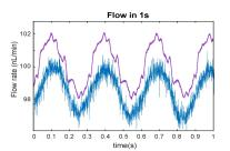
Comparison of extreme dynamic sensitivity of NIST flow meter with mechanically perturbed flow set nominal flow rate of 100 nL/min.
